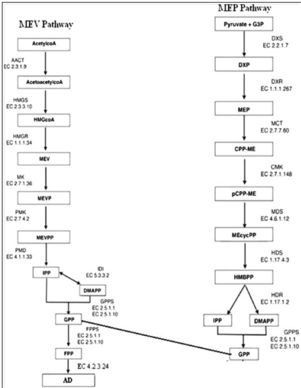
**Figure 6.7** Integrated MEV and MEP pathways for synthesis of AD. GPP flux from MEP pathway is directed towards MEV pathway which will successfully increase the FPP synthesis further it was converted to AD, an immediate precursor of artemisinin (Abbreviations are same as in Fig. 3)
