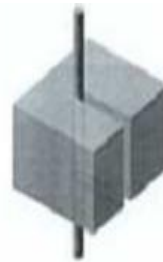
Figure 1.4: Single strand wire in work piece
