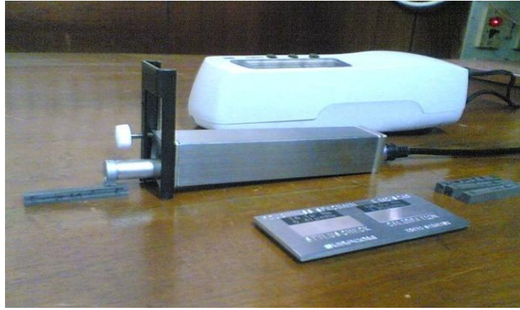
Figure 3.9: Setup to calculate Surface Roughness
