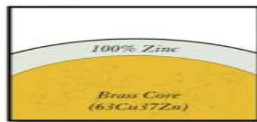
Figure 1.8: Zinc Coated Brass wire ( E_C )
