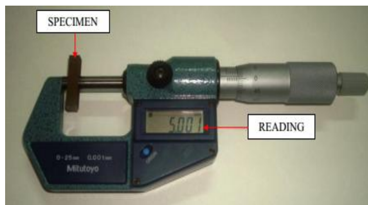
Figure 3.10: Setup for measurement of Dimensional Deviation
