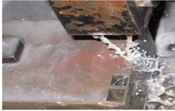
Figure 3.6: The Specimen Sample Machining Process of Wire EDM
