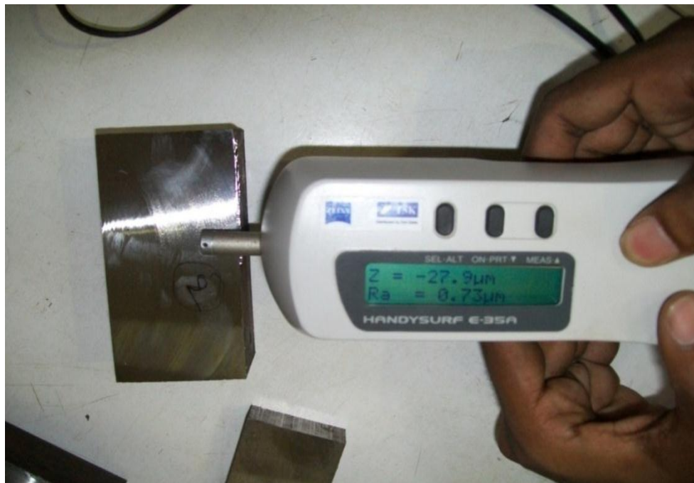
Figure 3.10 Measuring surface roughness using Handy surf
