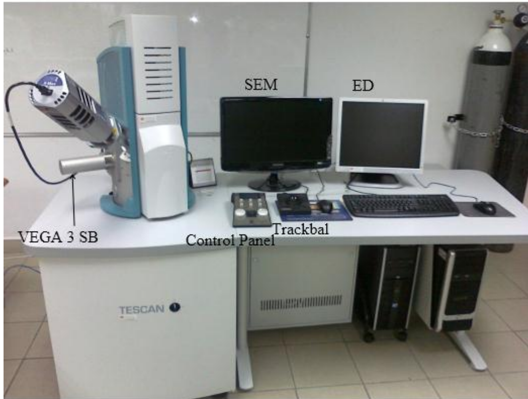
Figure 6.2 SEM and EDS Instrumentation and analysis Panel
