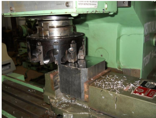
Figure 3.6 Face milling cutter body
