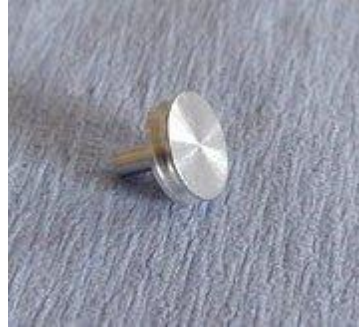
Figure 6.3 Standard specimen holder
