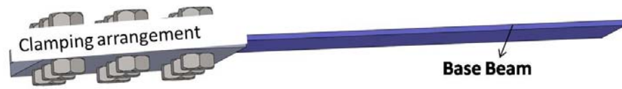
Figure 6.8 Schematic setup of base beam with clamping plate arrangement
