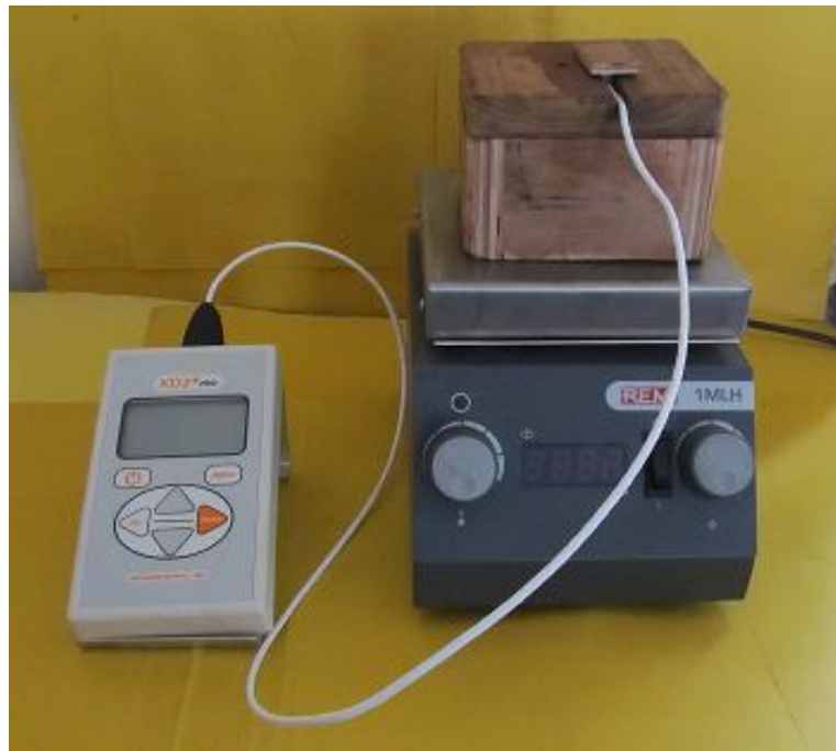
Figure 3.6: Experimental setup for measuring thermal conductivity at high temperatures
