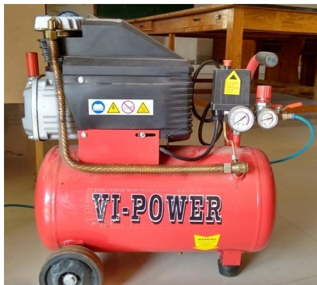
Figure 4.6: Compressor used for supply of pressurized air
