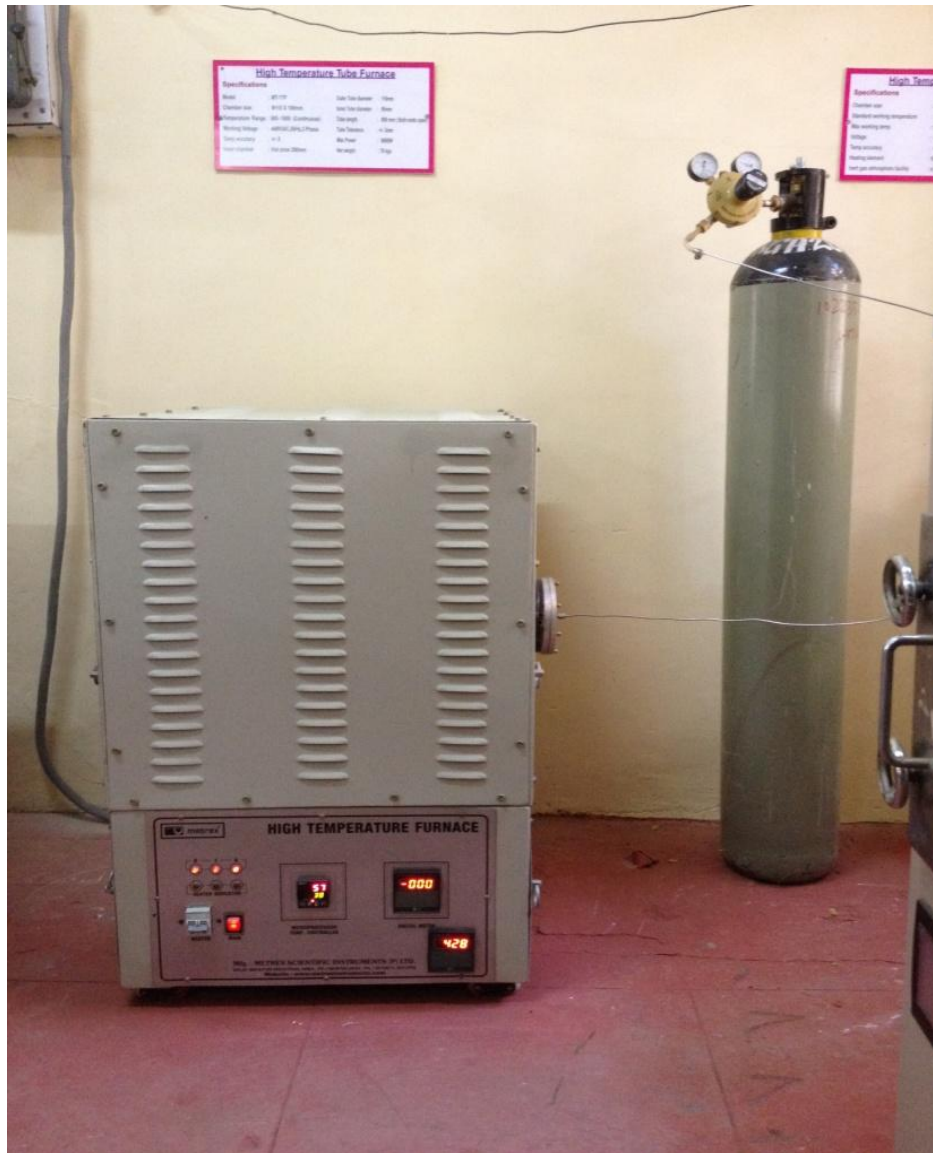
Figure 3.15. High-Temperature Tube Furnace.
