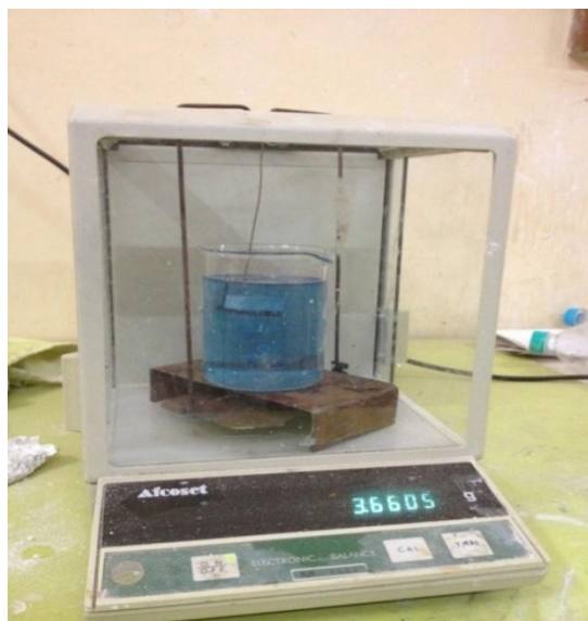
Figure 3.20. Electronic Analytical Precision Balance with Archimedes setup.
