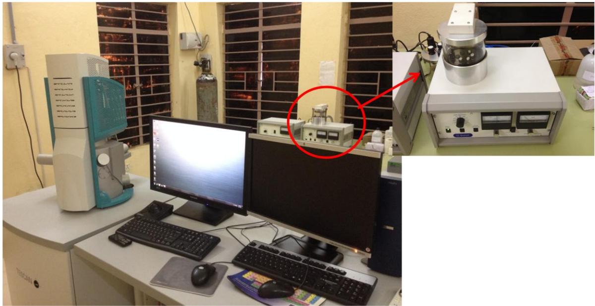
Figure 3.17. Scanning Electron Microscope with the sputtering setup.
