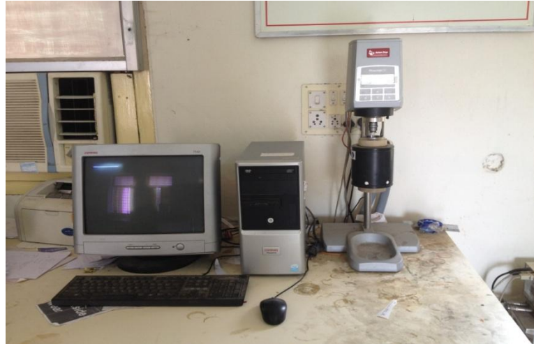
Figure 3.10. Setup showing computer controlled Rheometer
