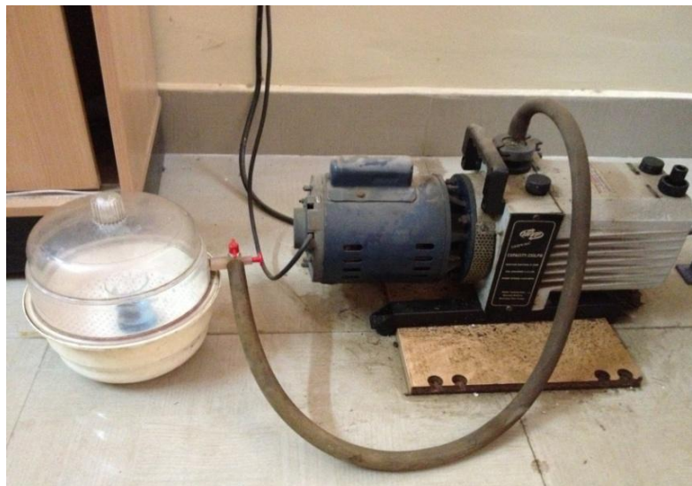
Figure 3.12. Desiccators with a vacuum pump.
