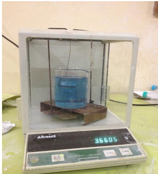
Figure 1.13. Schematic of Archimedes setup.
