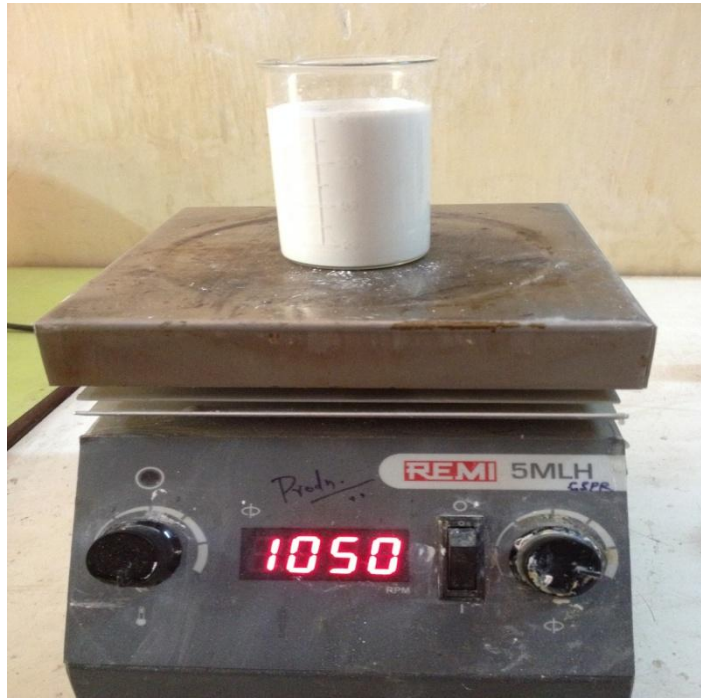
Figure 3.9. Magnetic stirrer setup
