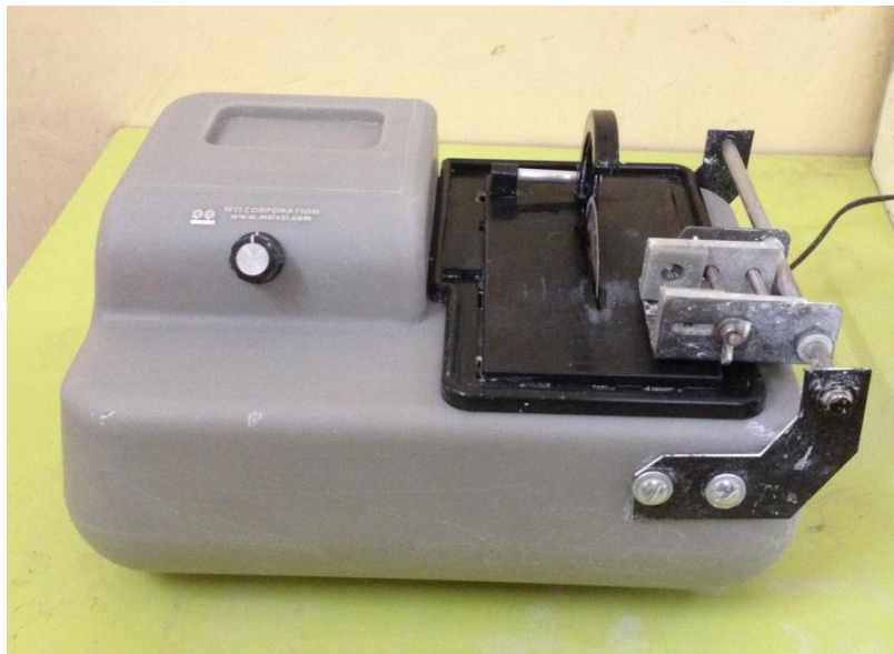
Figure 3.18. High-speed diamond cut-off saw.
