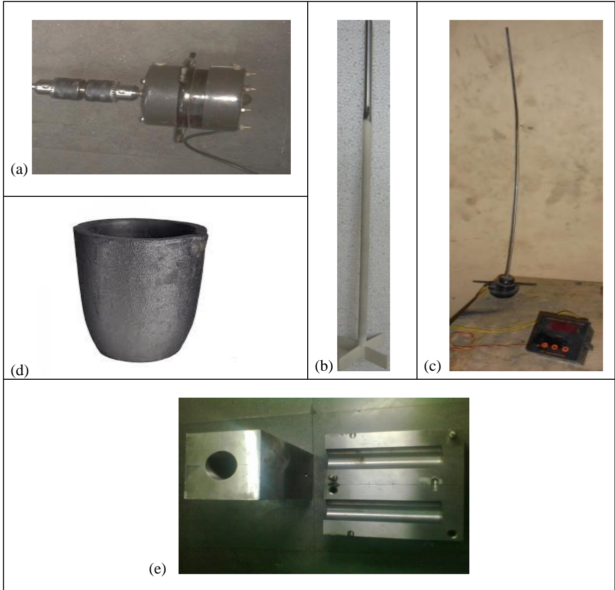
Figure 3.2: The photograph image of (a) Chuck attached to motor (b) SS 304 stirrer rod coated with Zirconia (c) K type Inconel temperature thermocouple (d) graphite crucible (e) stainless steel die
