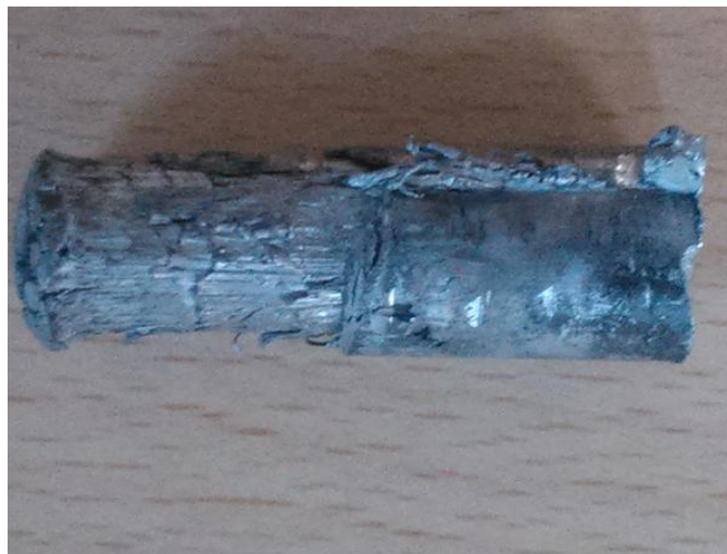
Fig.5.11 Thixo-extruded specimen cracked due to fluid segregation
