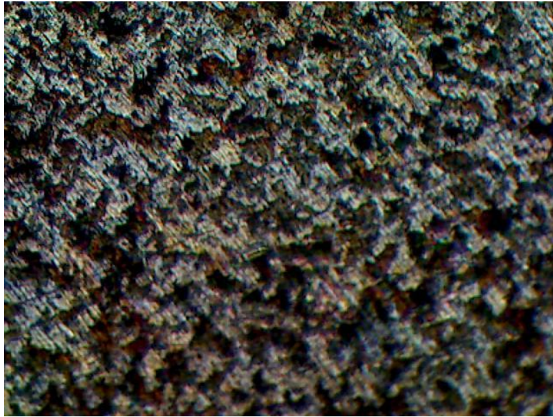
Fig. 3.2 Initial Microstructure of AA2017 aluminium sample
