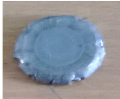
Fig. 4.6 Mushy state compressed sample at 610^{\circ}\text{C} and at a strain rate of 0.2\text{ s}^{-1}
