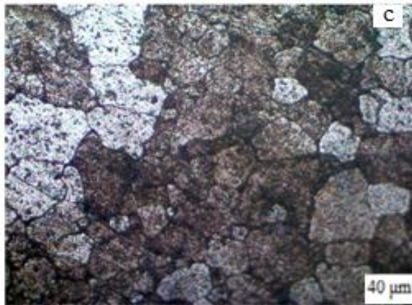
Fig.4.10 Microstructure of the samples compressed at different temperatures. (a) 570°C (b) 590°C (c) 610°C
