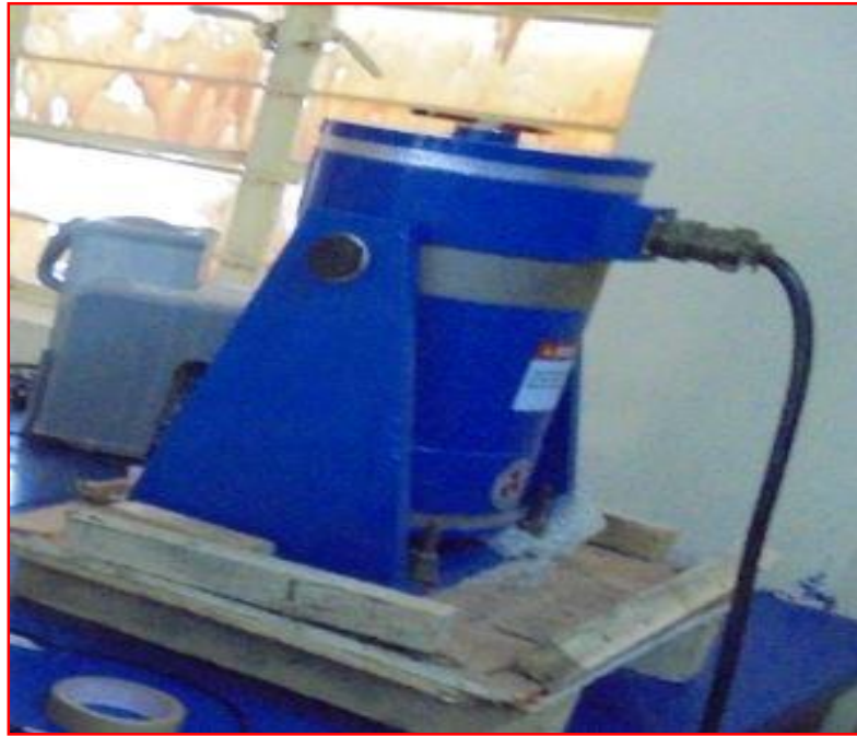
Fig.5.5 Electro dynamic exciter
