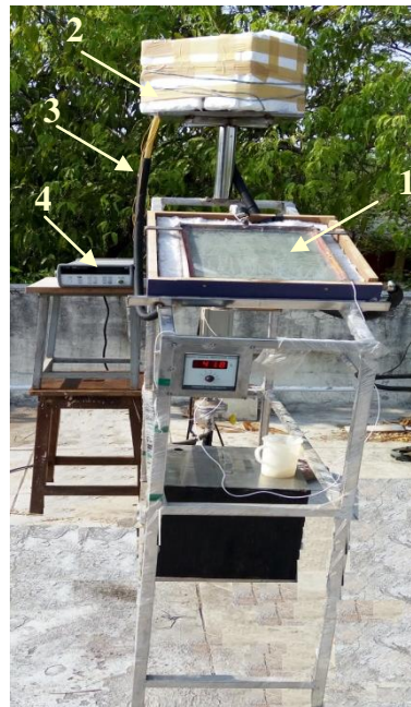
Fig. 4.48 Photographic view of NCDASFPC experimental test rig with temperature sensors
