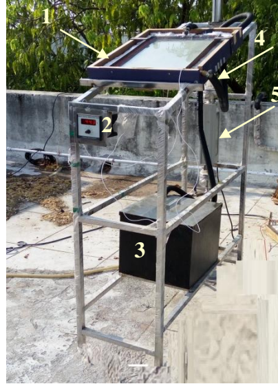
Fig. 4.21 Photographic view of FCDASFPC experimental test rig with mass flow meter and temperature sensors
