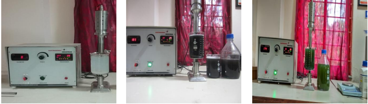
Fig 3.2. Preparation of nanofluids by ultrasonic sonicator (i) \text{Al}_2\text{O}_3 /water nanofluids (ii) CuO/water (iii) Cu/water
