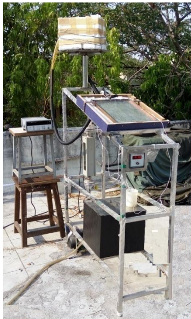
Fig. 4.48 Photographic view of NCDASFPC experimental test rig with temperature sensors
