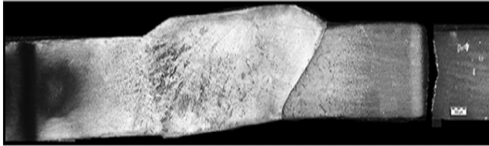
Fig. 4.2 Macrographs of fractured tensile test specimens of dissimilar welds of continuous TIG weld of Maraging steel and AISI 4130 steel.
