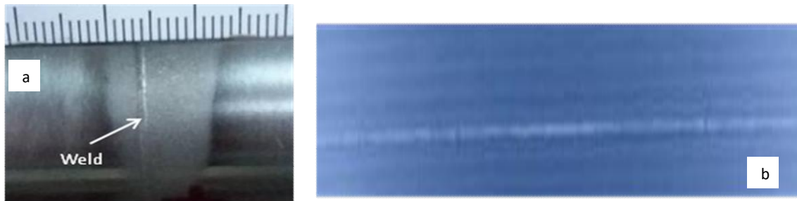
Fig 4.53 (a) Macrograph (top surface) and (b) X-radiograph of Laser beam welding of the Dissimilar steel i.e. Maraging steel to AISI 4130 steel.
