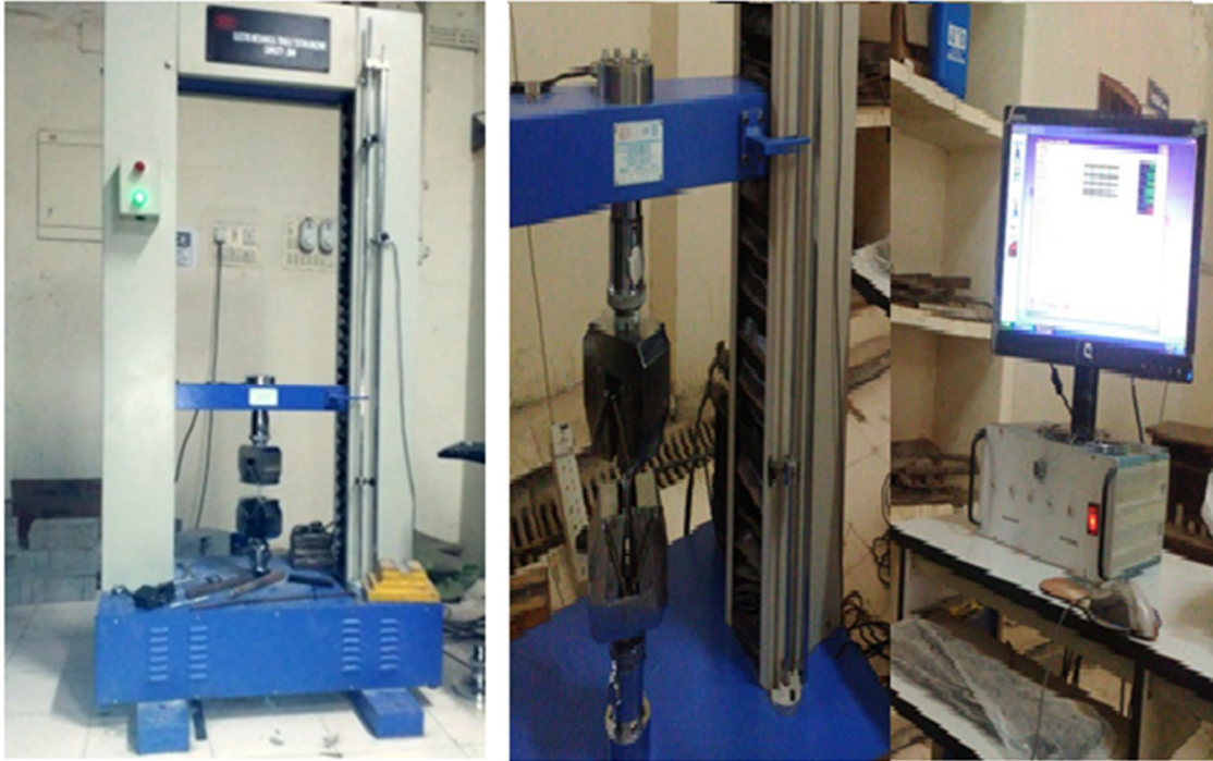
Figure 3.8 Electro Mechanical Tensile Test machine
