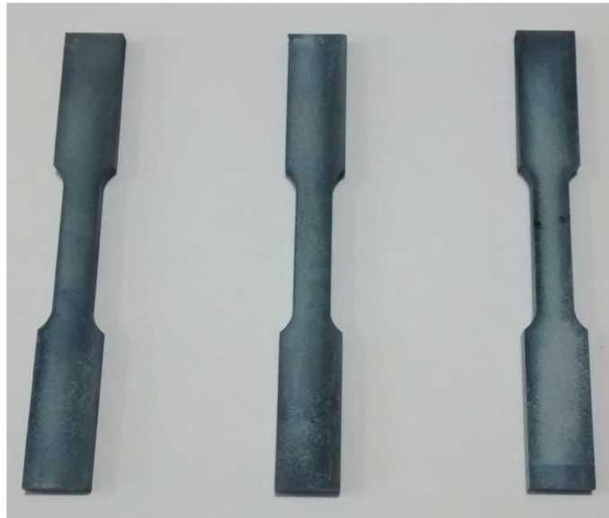
b) ZA-27 nanocomposites tensile samples
