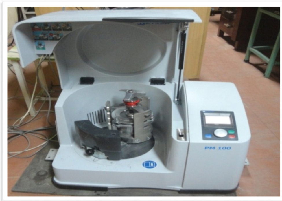
Figure.3.1 Planetary Ball Mill
