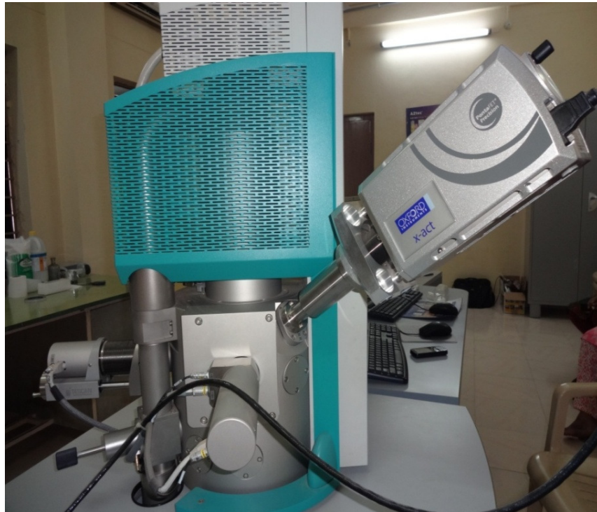
Figure 3.5 EDS coupled with SEM
