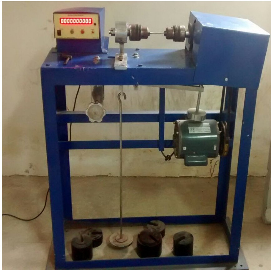
Figure 3.9 Rotating bending test machine
