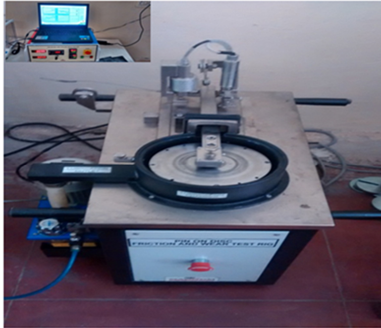
Figure 3.10 Pin on disc friction and wear testing machine
