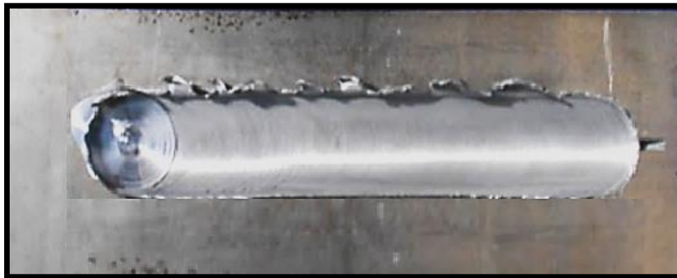
Fig. 4.1 Fabricated Al/Al 2 O 3 surface nanocomposite.
