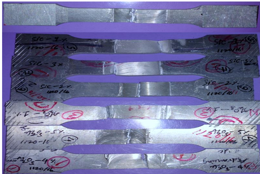
Fig. 4.27 Tensile tested samples of fabricated Al/Al 2 O 3 and Al/SiC.
