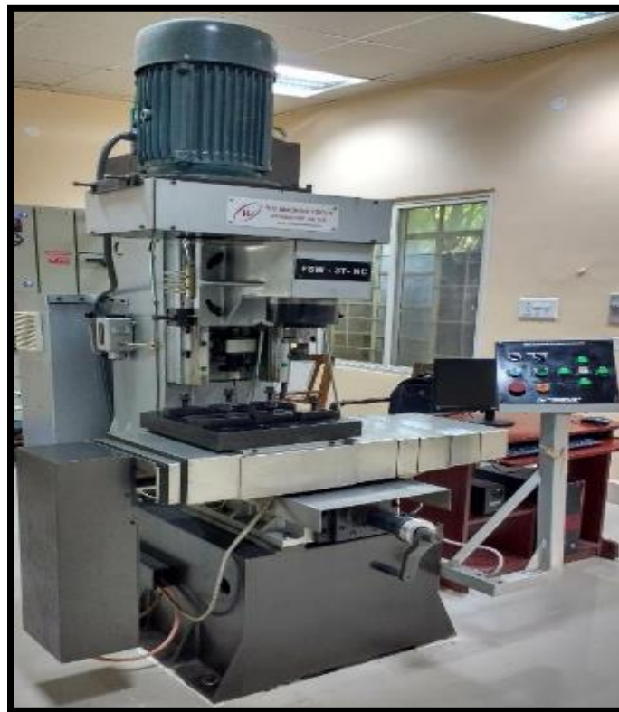
Fig. 3.3 Friction stir welding machine.
