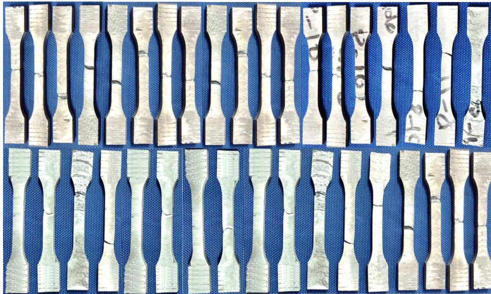
Fig. 4.48 Tensile tested samples of fabricated surface nanocomposites.
