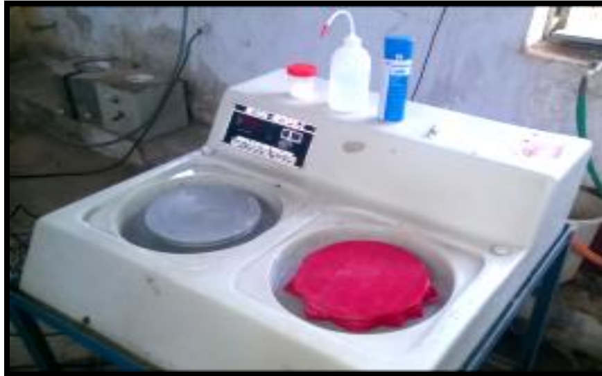
Fig. 3.8 Disc polishing machine.
