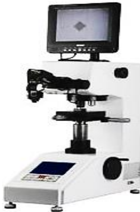
Fig. 3.16 Vicker's microhardness tester.
