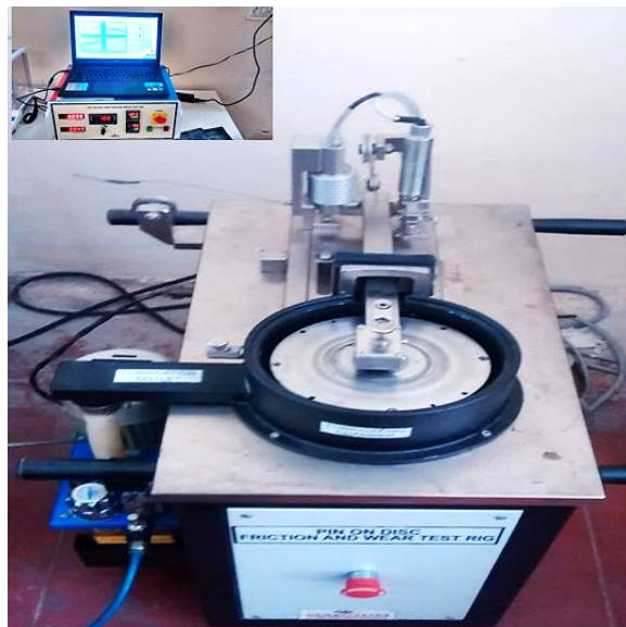
Fig. 3.19 Pin on disc friction and wear testing machine.
