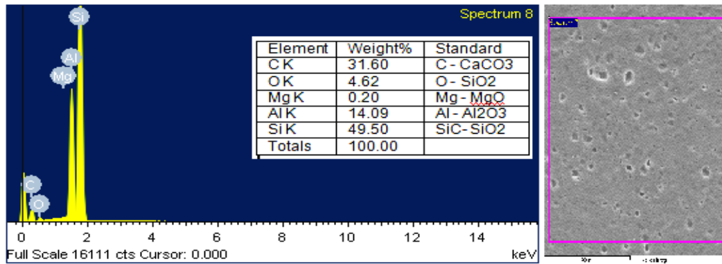
Fig. 4.22 EDS analysis of Al/SiC surface nanocomposite.
