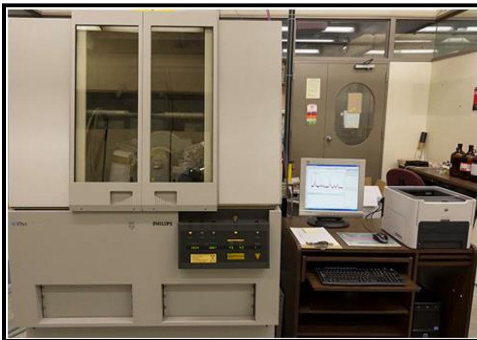
Fig. 3.12 Schematic diagram of X-Ray diffraction set-up.
