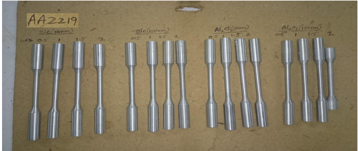
Figure 3.9 Tensile testing specimens of AA 2014 & AA 2219/SiC (150 nm, 50 nm), AA 2014&AA 2219/Al 2 O 3 (150 nm, 50 nm)
