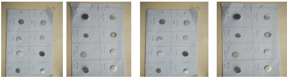
Figure 3.10 Hardness specimens of AA 2014 & AA 2219/SiC (150 nm, 50 nm), AA 2014&AA 2219/Al 2 O 3 (150 nm, 50 nm).
