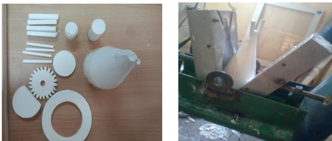
Figure 3. 16: (a) Typical shaped samples (b) A green radome after gelation in the mould.
