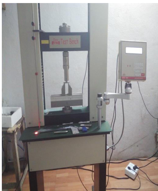
Figure 3. 8: Universal Testing Machine
