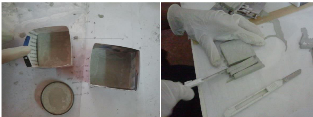
Figure 3. 4: (a) Moulds and (b) samples cutting after gelation process
