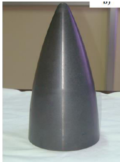
Figure 1. 2: Photograph of sintered and machined \text{Si}_4\text{Al}_2\text{O}_2\text{N}_6 radome [9]
