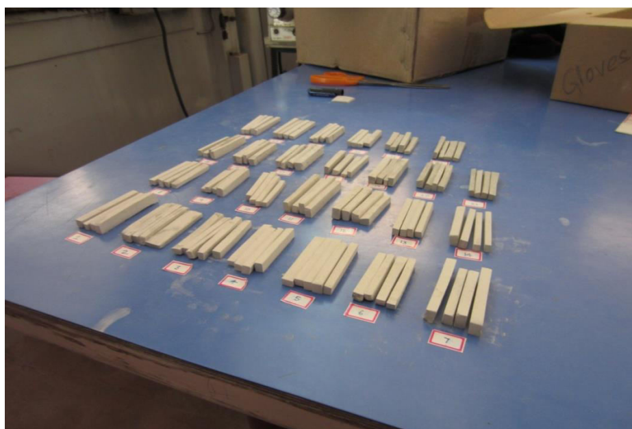
Figure 3. 17 Sintered \text{Si}_3\text{N}_4 - \text{SiO}_2 -BN samples for flexural strength measurement
