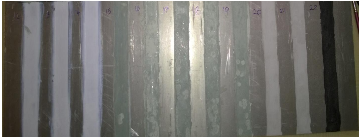
Figure 3.9: illustrates the painting of mixture of ceramic powders and poly-vinyl-alcohol in the prepared grooves.
