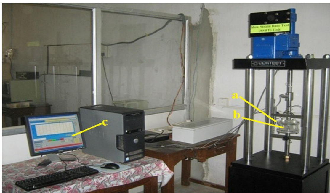
Figure 3.3: Slow Strain Rate Test unit. (a) Extensometers (b) vessel carrying corrosive media (c) Computer attachment to record deformation data
