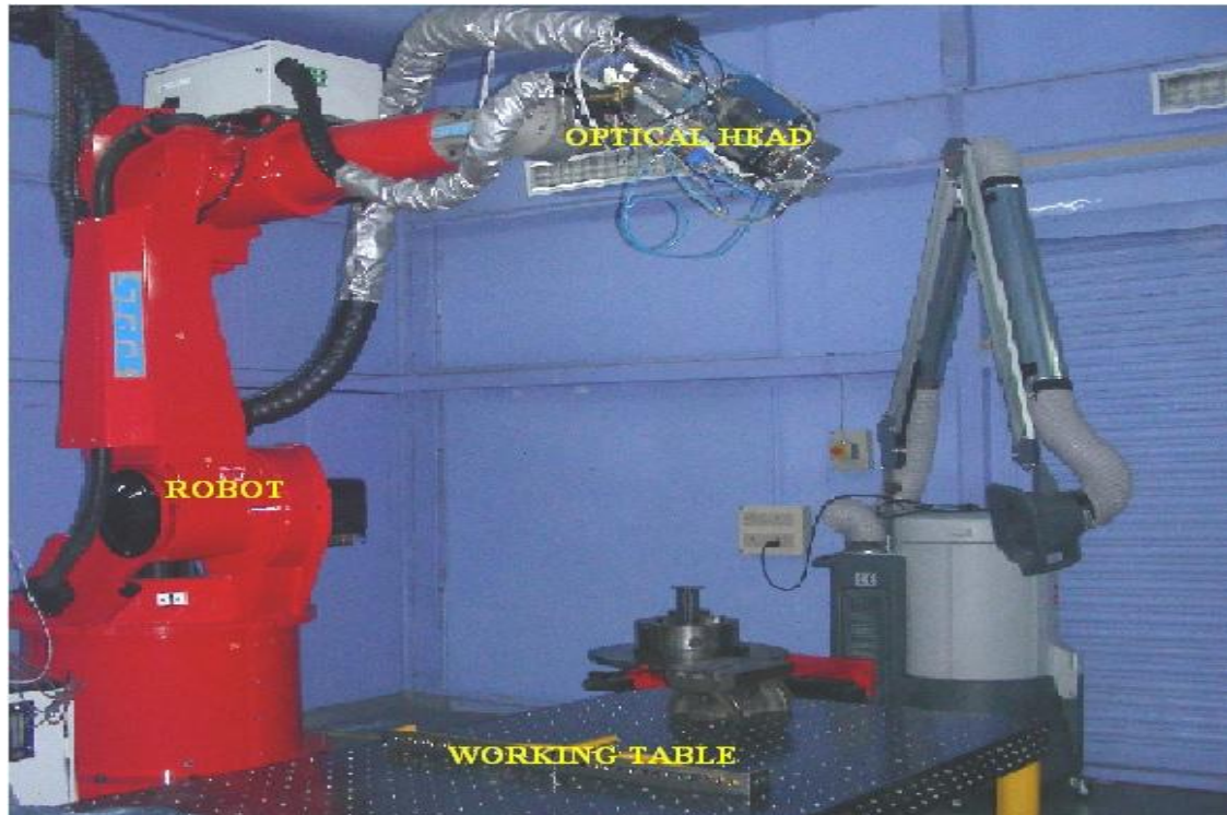
Figure 3.5: Laser processing setup utilized for experimentation
