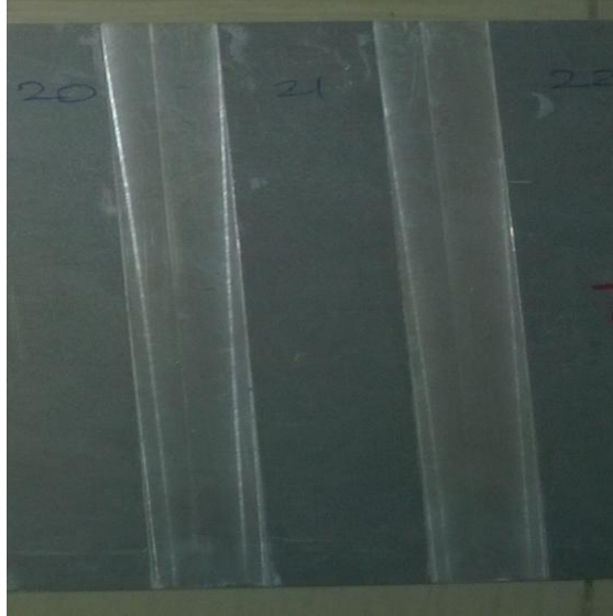
Figure 3.8: illustrate the grooves prepared on the 7075 Al alloy prior to the coating of powders.
