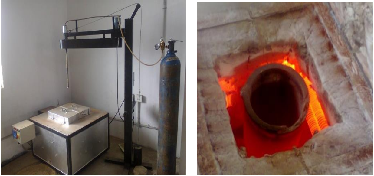
Figure 1.8: a) Stir casting equipment b) Crucible inside the stir casting furnace
