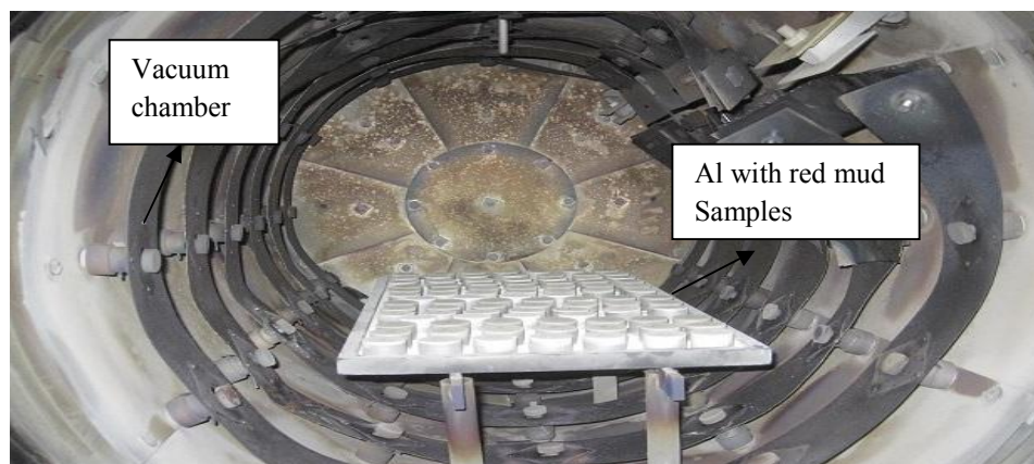
Figure 3.13: Compacted Pure Aluminium and Red mud samples in Sintering Furnace
