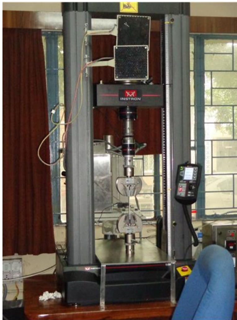
Figure 3.12 INSTRON 5967 tensile testing machine: test specimen fitted with extensometer
