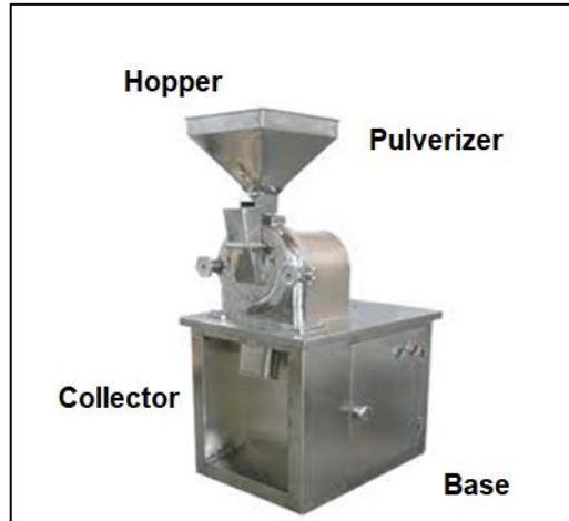
Figure 3.2. Pulverizer used for breaking agglomerates and mixing of the powders
