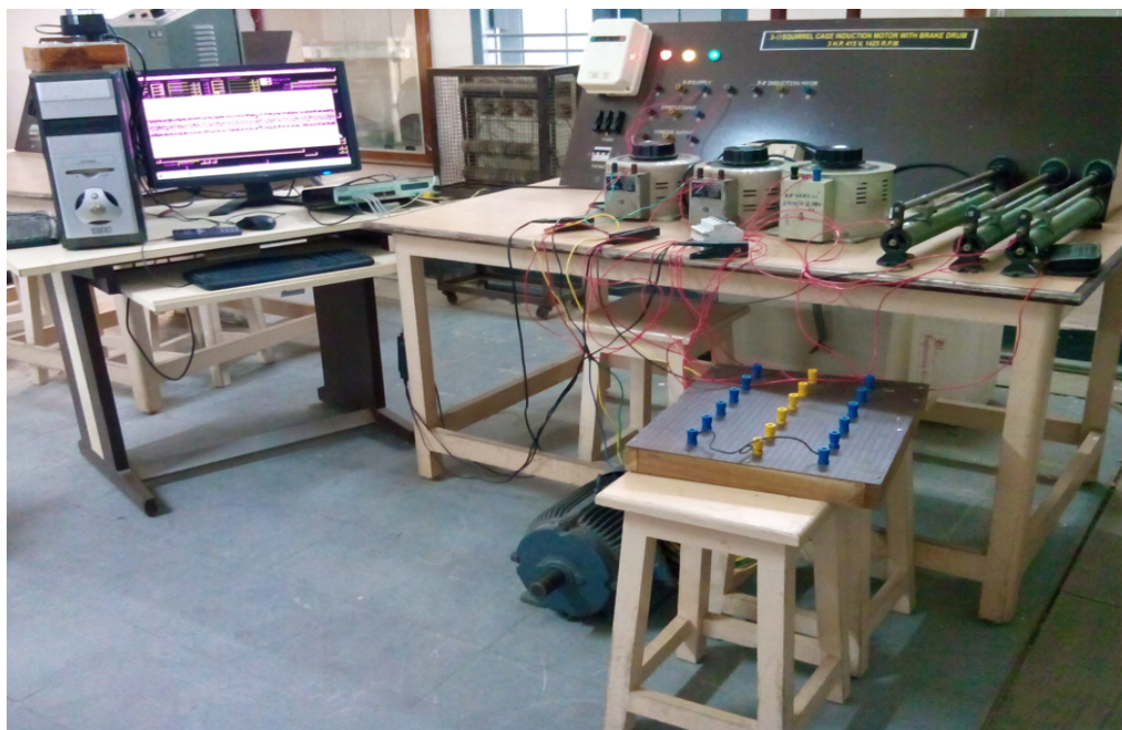
Figure 3.40: Experimental setup for 10-hp induction motor
