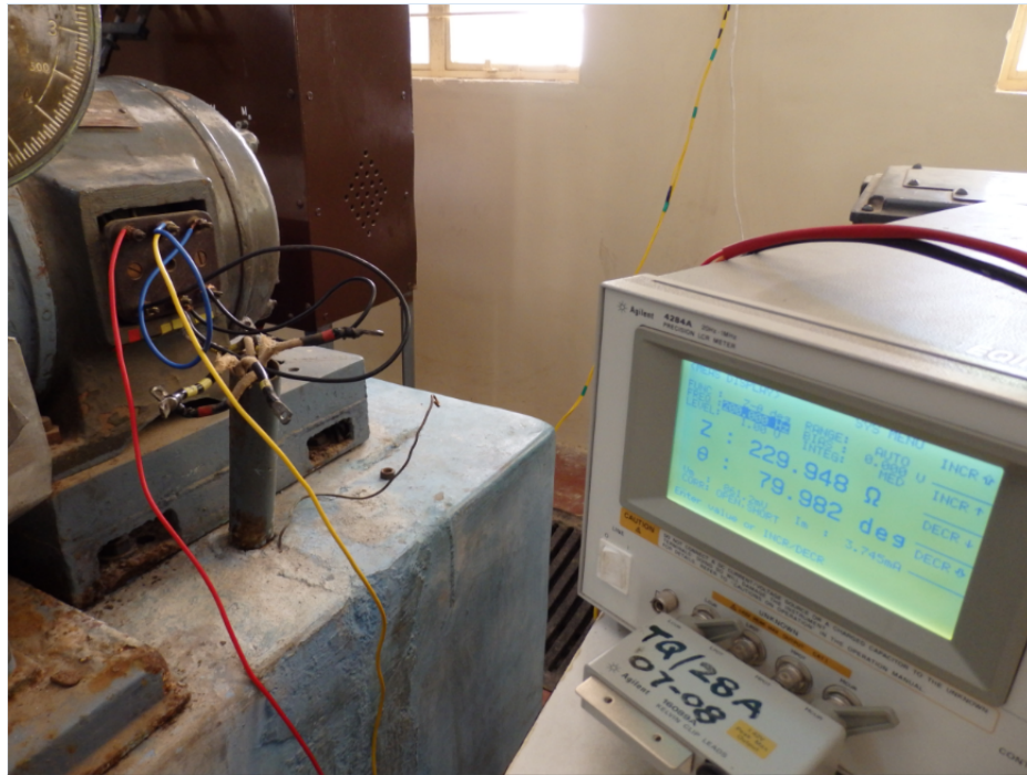
Figure 2.6: Experimental setup for DM test on a 3-phase, 5-hp induction motor
