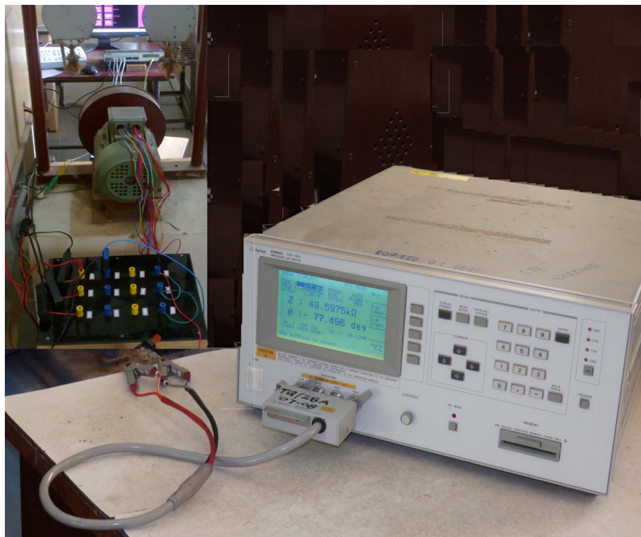
Figure 2.8: Experimental setup for a 3-phase, 3-hp induction motor
