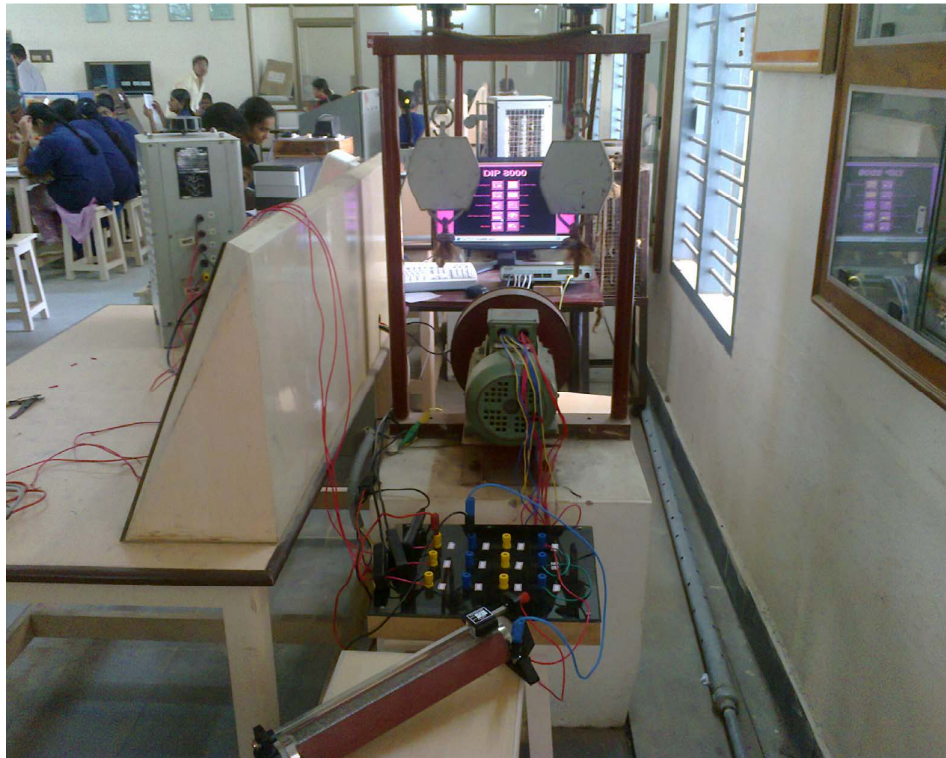
Figure 3.39: Experimental setup for 3-hp induction motor
