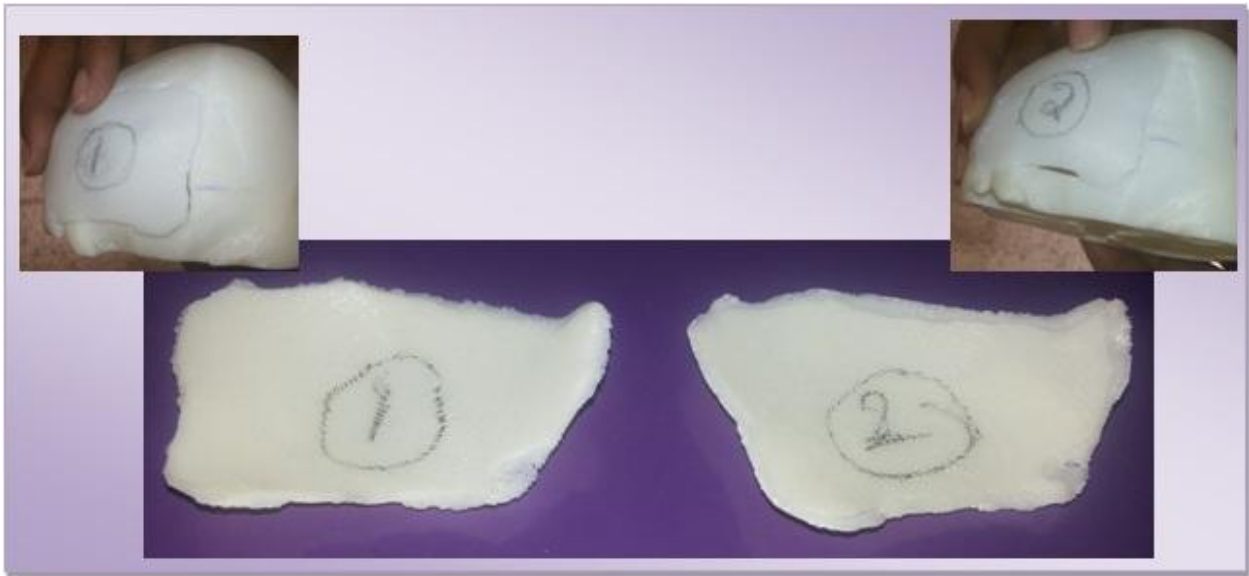
Figure 3.8 Final product 1) Chamfered edges with max clearance 2) Modified chamfered edges with less clearance
