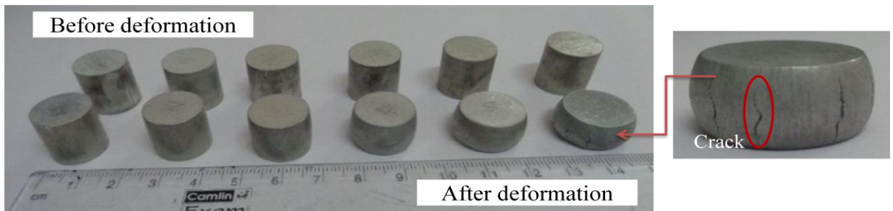
Fig. 3.12 Photograph of preforms before and after deformation test
