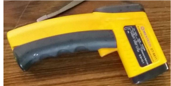
Figure: 4.10 Working Principle of IR Thermometer Figure: 4.11 Infrared thermometers (IR)
