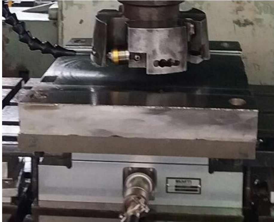
Fig.2.4. Diagram showing rotary milling cutter and work piece interaction
