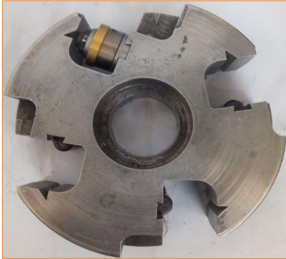
Fig.3.15. Photograph of the developed rotary milling cutter with four inclination angles
