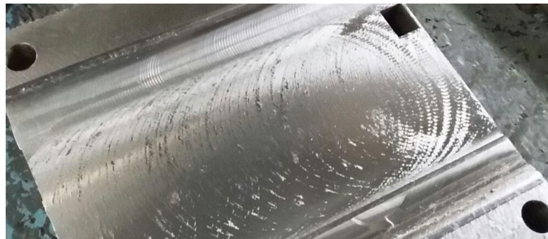
Fig.5.3.1.2 Surface roughness pattern generated in rotary face milling
