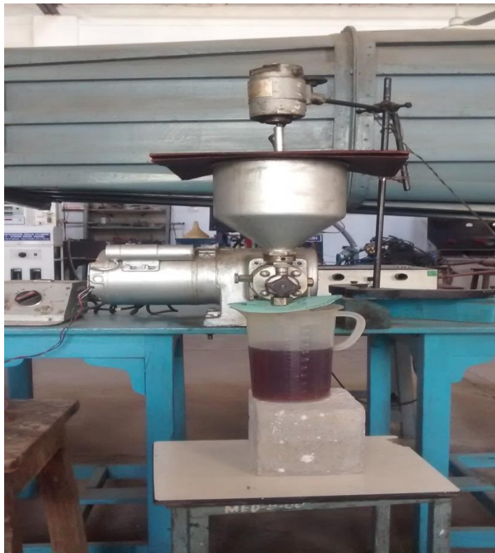
Fig. 3.5. PPO blends preparation by using Emulsifier Apparatus.
