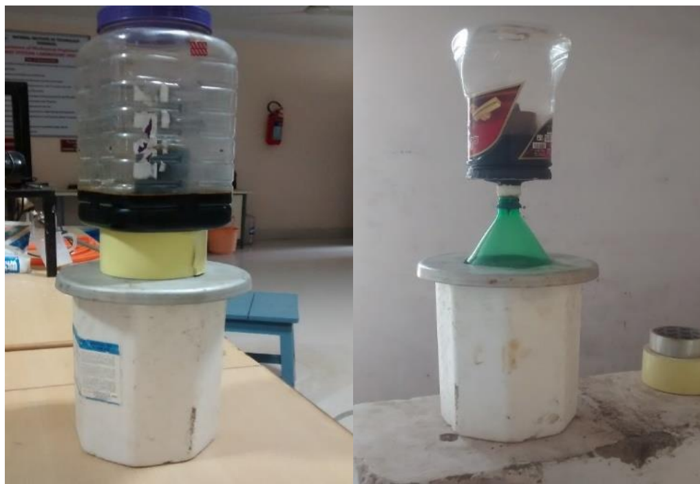
Fig. 3.6. Primary (cloth) and secondary (coil) filtration process
