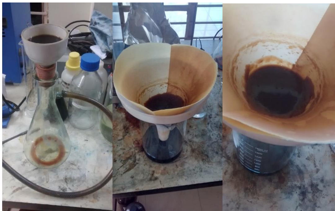
Fig. 3.10. Nano and Micro filtration process of crude PPO after cavitation
