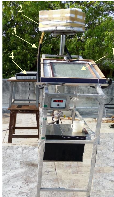
Fig. 5.15 Photographic view of NCDASFPC experimental test rig with temperature sensors
