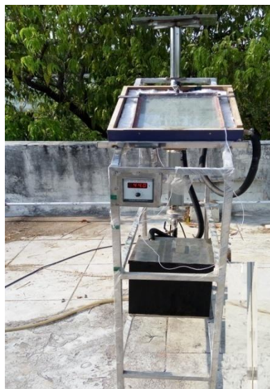
Fig. 4.21 Photographic view of FCDASFPC experimental test rig with mass flow meter and temperature sensors
