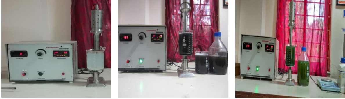
Fig 3.1. Preparation of nanofluids by ultrasonic sonicator (i) \text{Al}_2\text{O}_3 /water nanofluids (ii) CuO/water (iii) Cu/water
