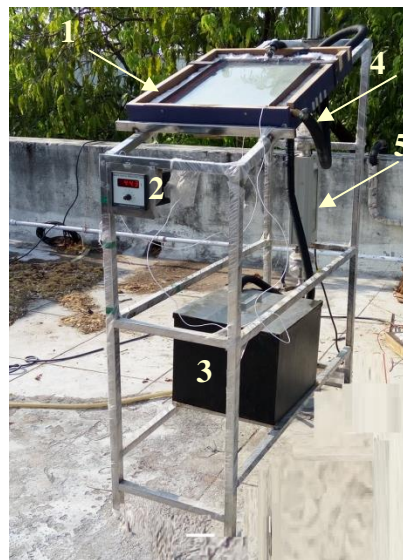
Fig. 4.21 Photographic view of FCDASFPC experimental test rig with mass flow meter and temperature sensors
