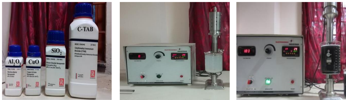
Fig 3.2. Preparation of nanofluids by ultra-sonicator (i) \text{Al}_2\text{O}_3 , \text{CuO} , \text{SiO}_2 nanopowder and C-TAB surfactant (ii) \text{Al}_2\text{O}_3 -water nanofluid (iii) \text{CuO} -water nanofluid
