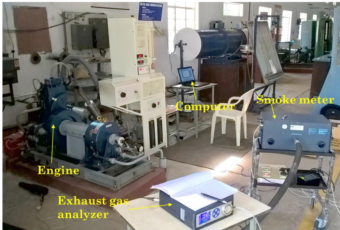
Fig. 3.8 Experimental setup of the VCR engine
