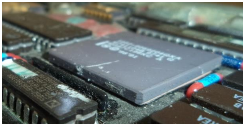
Figure 3.11 SMT with Gap
