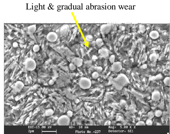
Fig.2.3: SEM micrograph of ASP 30 [48]
