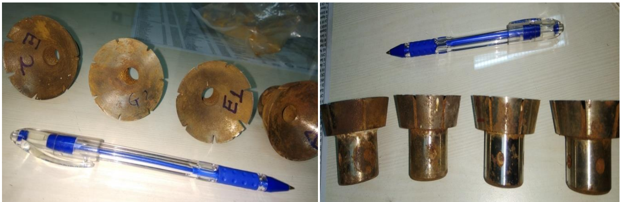
(a) Corrosive damage on rake face of the inserts (b) Corrosive damage on flank face of inserts
