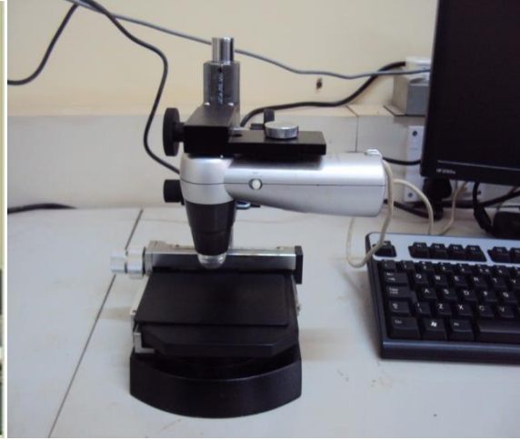
Fig. 6.5: USB digital Micro scope for chip morphology Study (Capacity: 2000x)
