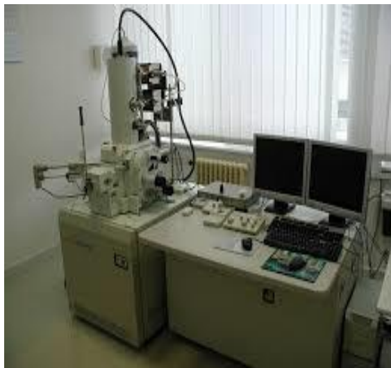
a) Metallographic microscope(GX71, Olympus) b) Scanning Electron Microscope(JOEL JSM - 6610LV)
