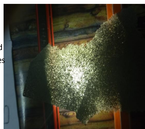
(d) See through holes in thin chip of propellant
