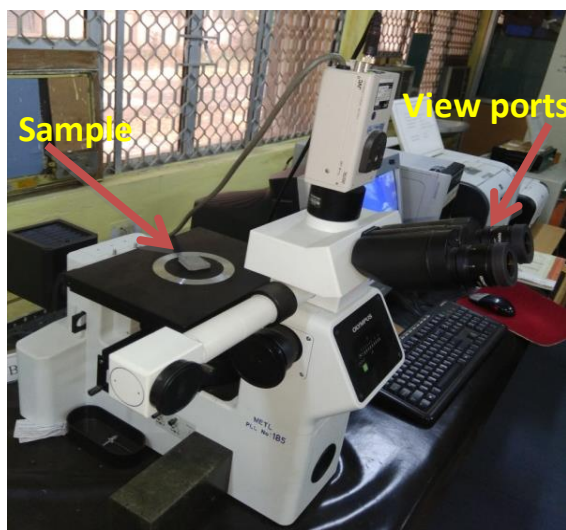
a) Metallographic microscope(GX71, Olympus) b) Scanning Electron Microscope(JOEL JSM - 6610LV)
