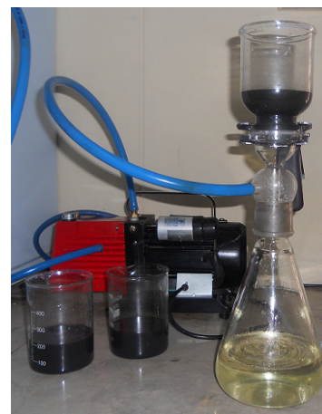
Fig 3.3. Vacuum filtration setup
