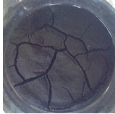
Fig 3.5. Solid lumps obtained after drying
