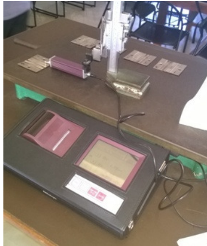
Fig 3.17. Mitutoyo SJ 310 surface roughness testing equipment
