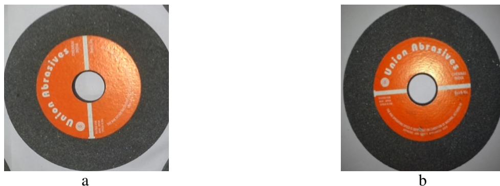
Fig 3.7.D (a) Standard Grinding Wheel (b) GNP impregnated grinding wheel
