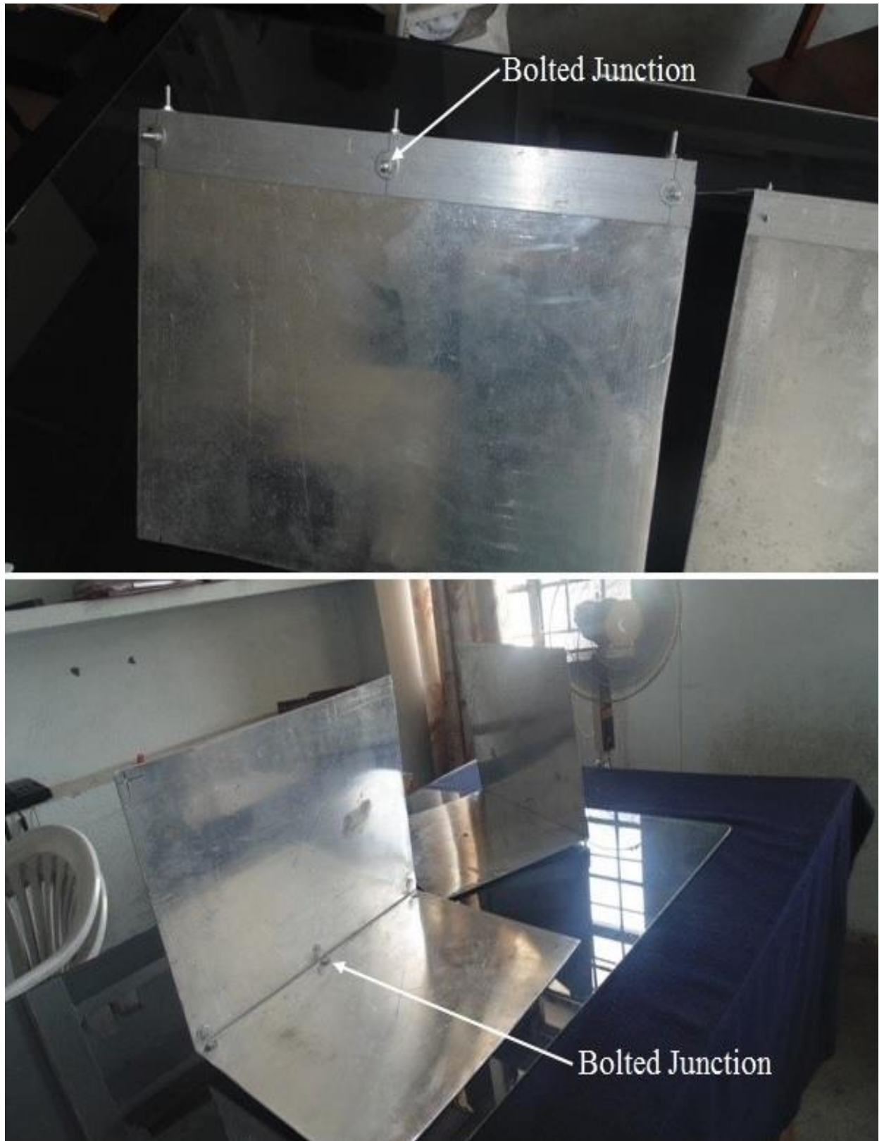
Figure 6.18 Bolted junctions for aluminium plates
