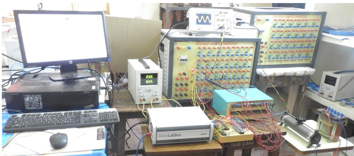
Fig. A.7: The experimental set-up with dSPACE RTI1202 controller.
