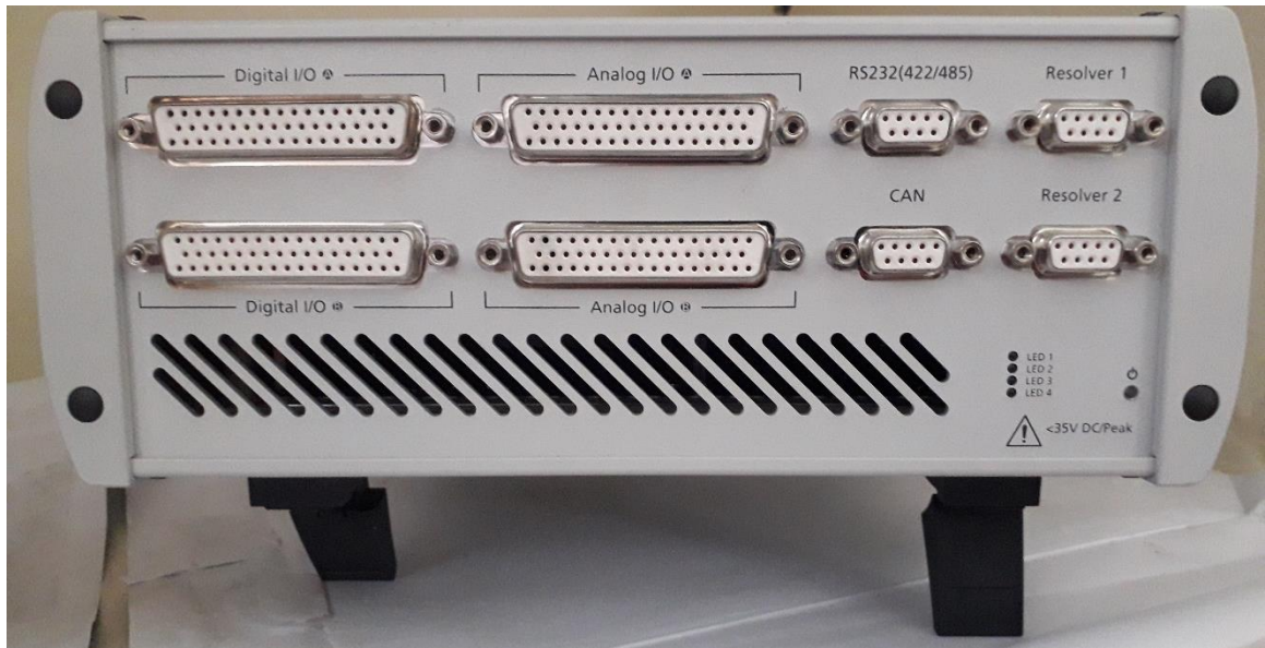
Fig. A.5: Digital I/Os of dSPACE-RTI1202 controller.
