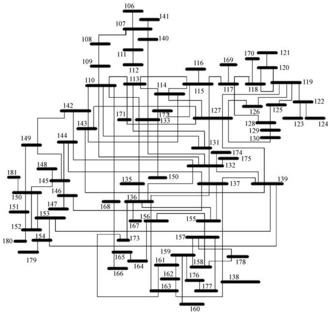
Figure A.2: Single line diagram of Andhra Pradesh state regional grid
