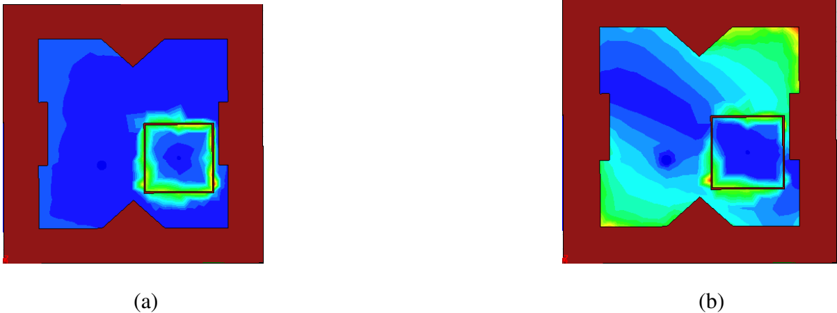
Fig. 3.13 Simulated surface current distribution (a) at 2.4 GHz (b) at 3.25 GHz
