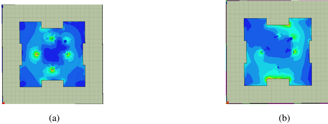
Fig. 4.4 Simulated surface current distribution (a) at 2.4 GHz (b) at 3.4 GHz
