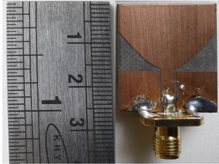
Figure 3.15 The fabricated curvature profile monopole antenna
