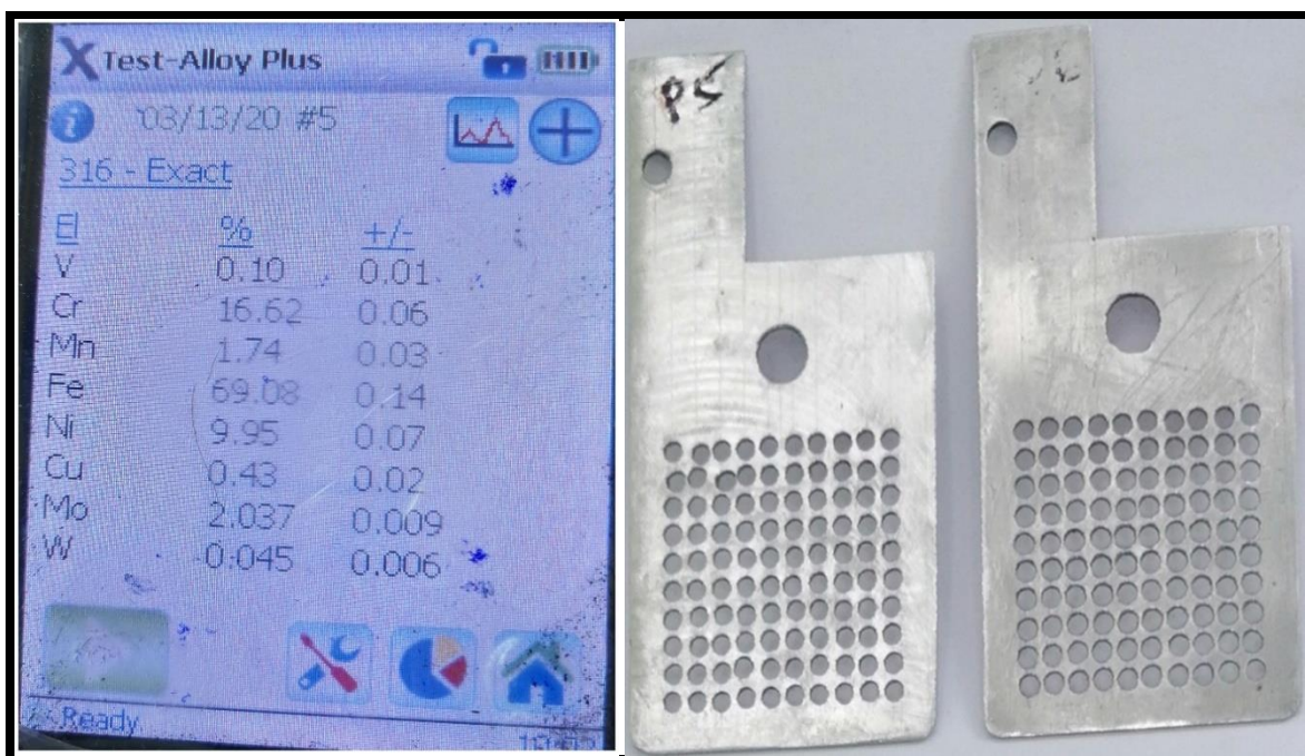
Figure 3.11 Details of SS-316L material and Fabrication of uniform cylindrical openings on current collectors
