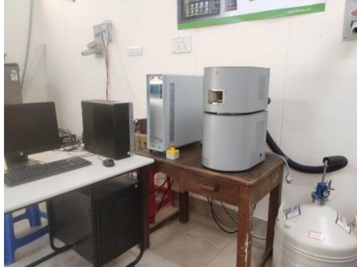
Fig. 3.4. Damping setup for measuring damping capacity
