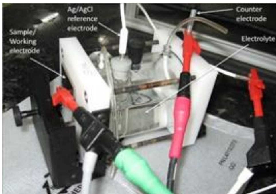
Fig. 3.3 Electrochemical setup for corrosion test
