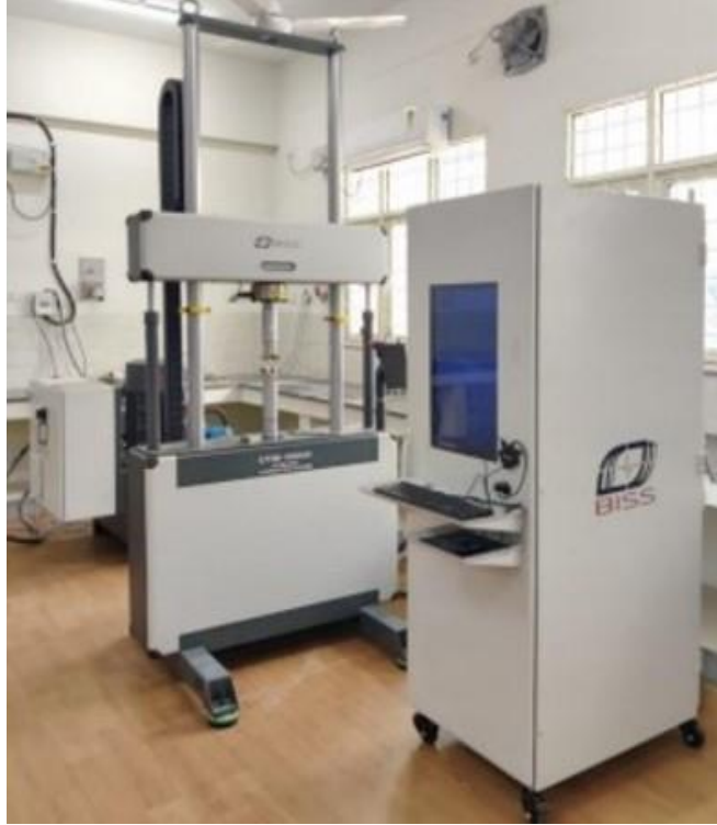
Fig. 3.5. Fatigue testing setup to measure fatigue crack growth rate
