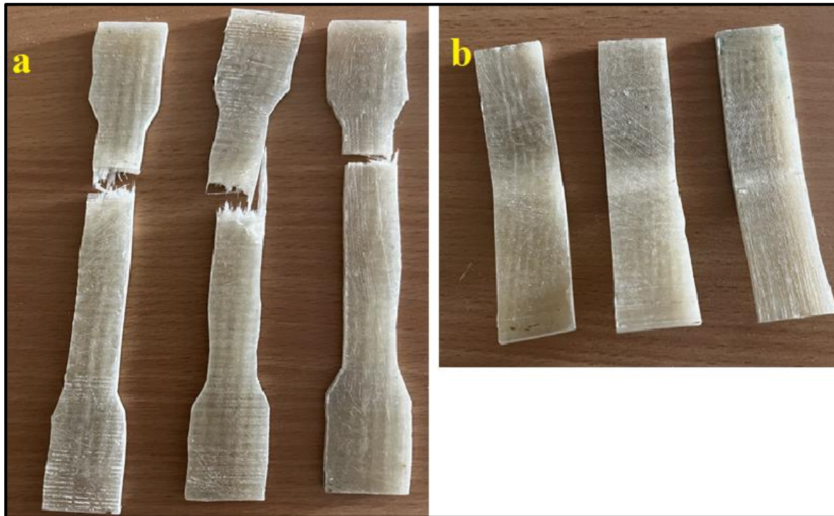
Figure 3.9 Shows the samples after testing a) Tensile b) Flexural
