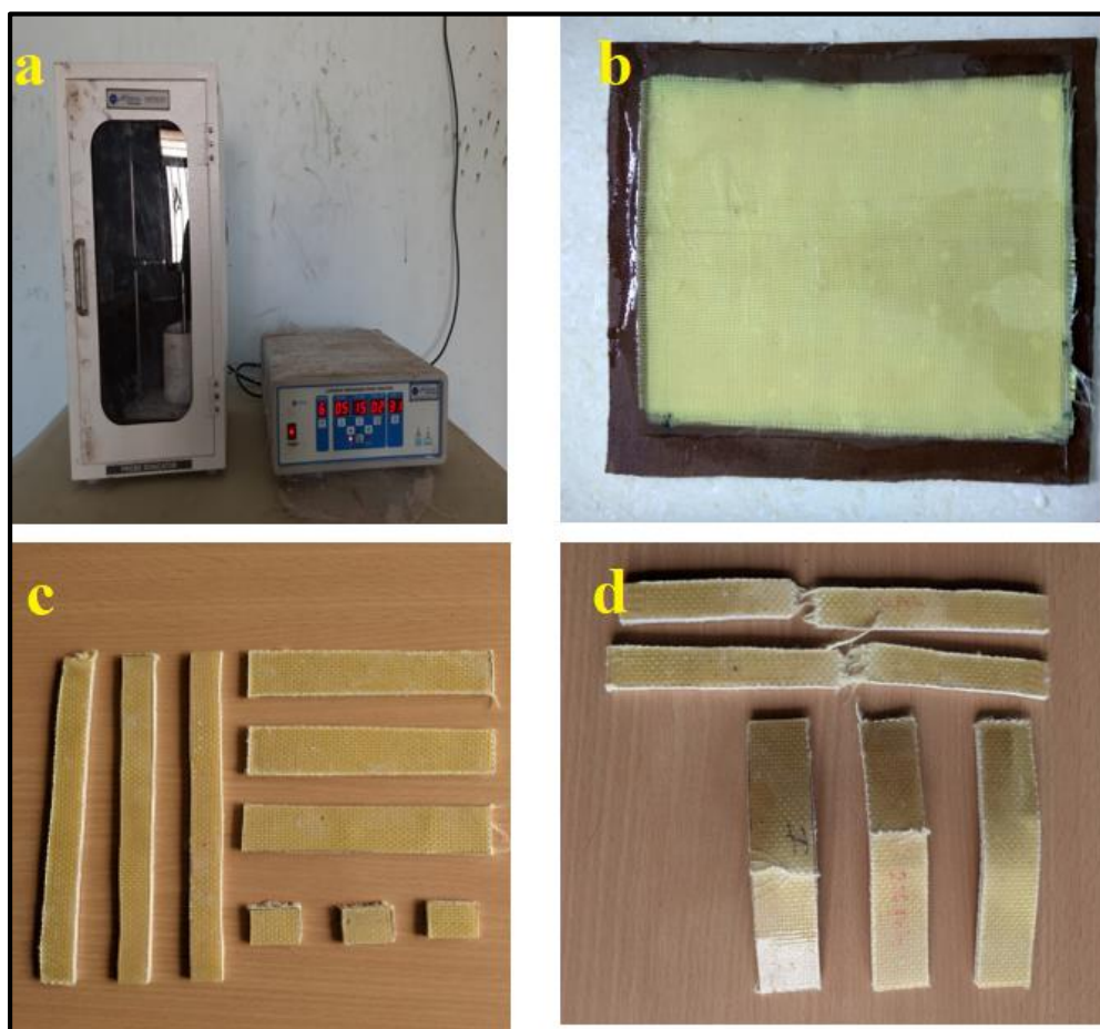
Figure 4.4 Shows the sample preparation step by step procedure
