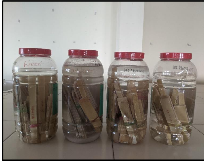
Figure 5.2. Shows the mechanical samples immersed in various environments
