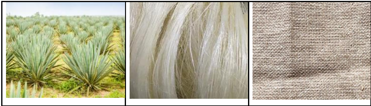
Figure 1.2. Sisal fiber and Sisal fiber after extraction (Continuous and Mat form)
