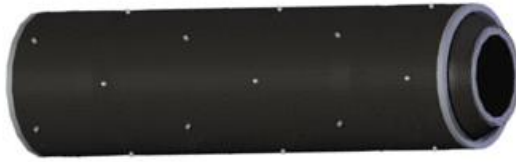
Figure 5.9. Distribution of Sensors over a Typical Rocket Motor.
