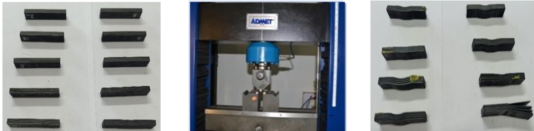
Figure 3.21. ILSS Test (a) Test Specimen (b) Test Setup (c) Failed Specimens.
