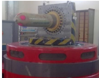
Figure 6.5. Test Set-up for Random Vibration.
