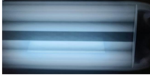
Figure 7.7. RT of SRM with Composite Case (after 60 ISAT B Cycles)
