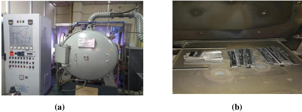
Figure 3.11. (a) Moisture Removal Chamber (b) Samples inside the Chamber.
