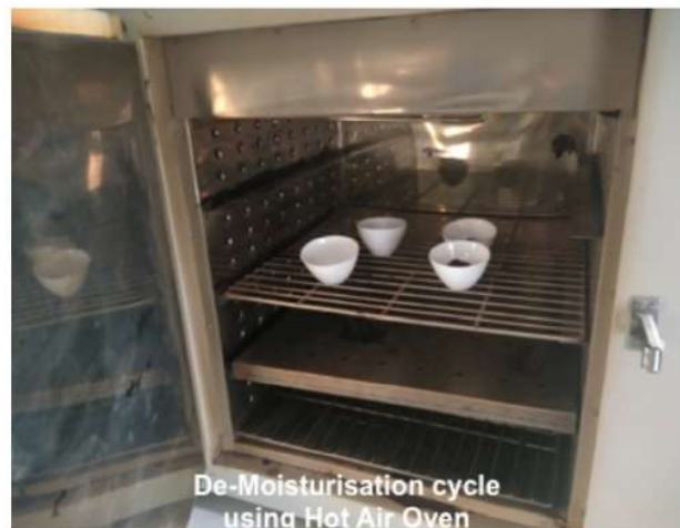
Fig. 4.2 De-moisturization cycle using hot air oven
