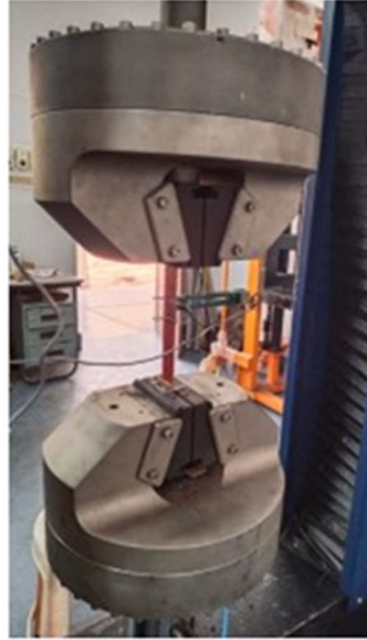
Fig. 6.41 Test specimen undergoing IPSS test
