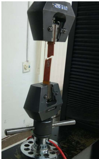
Fig. 3.18 Test specimen undergoing IPSS test
