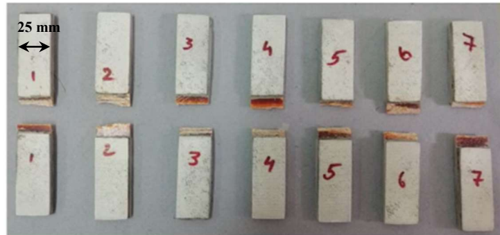
Fig. 3.12 Fractured specimen after compression test
