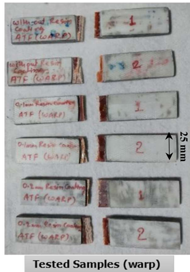
Fig. 6.7 Compressive strength (warp) test samples after ATF exposure (after testing)
