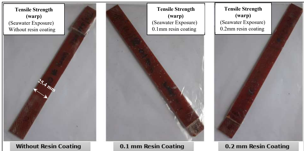
Fig. 6.28 Test samples of the tensile strength (warp) after seawater exposure (after testing)
