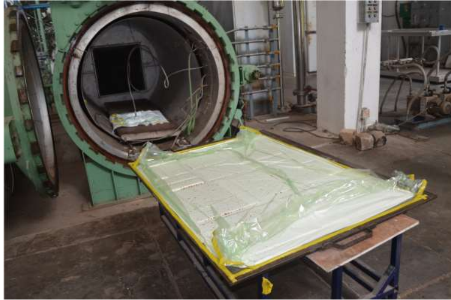
Fig. 3.2 Curing of test laminates in the autoclave
