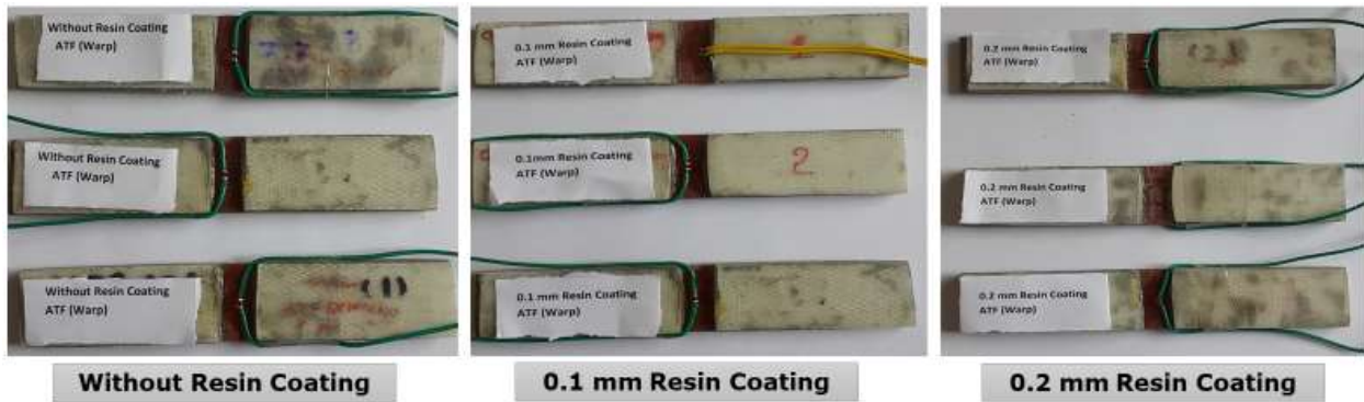
Fig.6.5 Test samples of compressive strength (warp) after ATF exposure (before testing)
