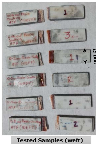
Fig. 6.10 Compressive strength (weft) test samples after ATF exposure (after testing)
