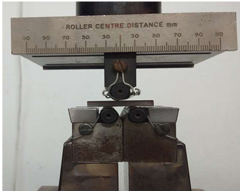
Fig. 3.15 Test specimen undergoing ILSS test
