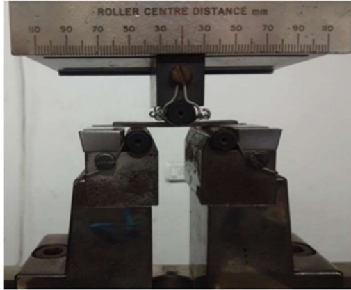
Fig. 3.13 Test specimen undergoing flexural test
