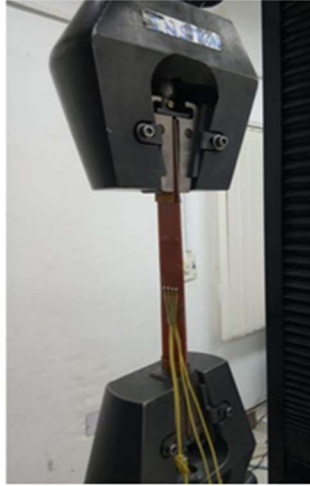
Fig. 3.9 Test specimen undergoing tensile test
