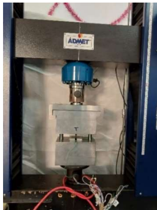
Fig. 3.11 Test specimen undergoing compression test
