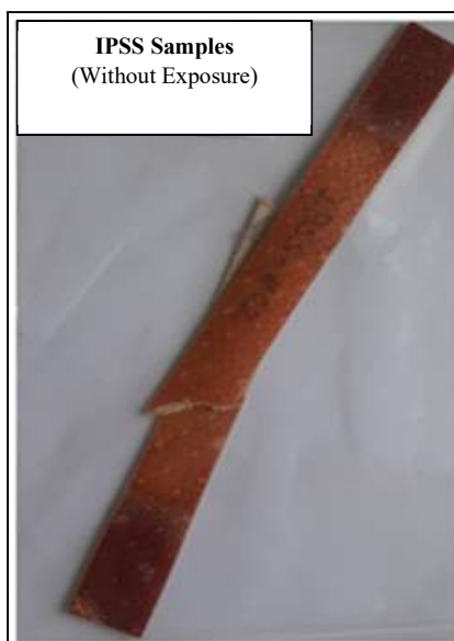
Fig. 3.19 Fractured specimen after IPSS test
