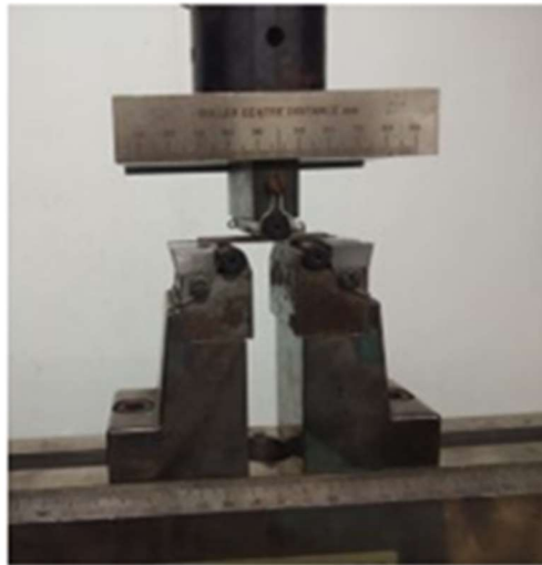
Fig. 6.34 Test specimen undergoing flexural test
