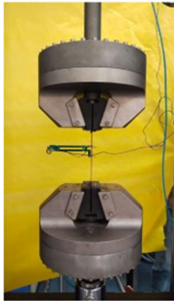
Fig. 6.26 Test specimen undergoing tensile test
