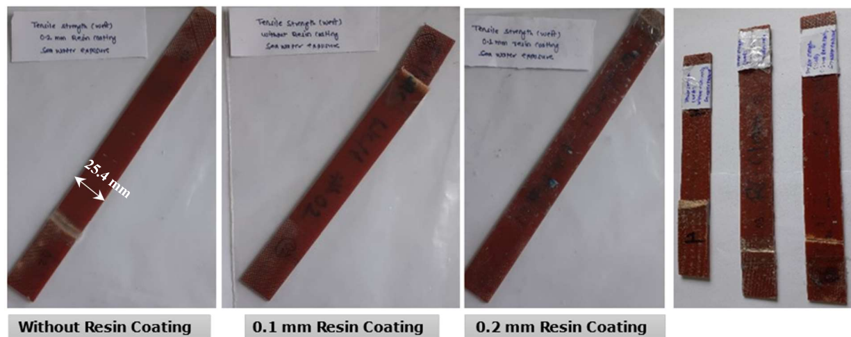
Fig. 6.30 Test samples of the tensile strength (weft) after seawater exposure (after testing)
