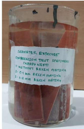
Fig. 5.4 Test samples of compressive strength (warp and weft) immersed to seawater exposure
