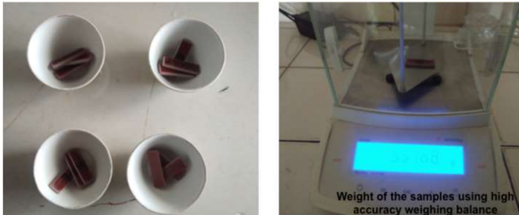
Fig. 4.1 ILSS and flexural test samples (before de-moisturization)
