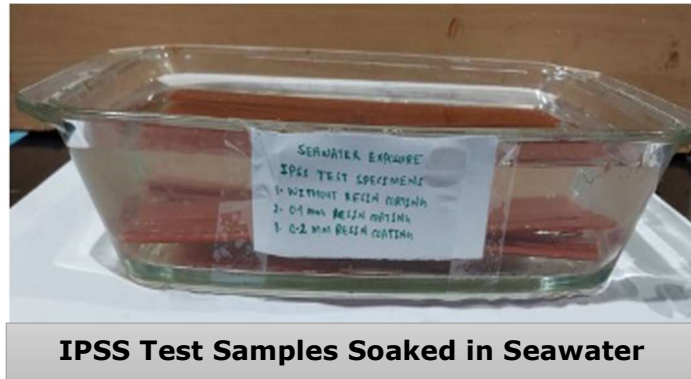
Fig. 5.13 IPSS test samples immersed in seawater
