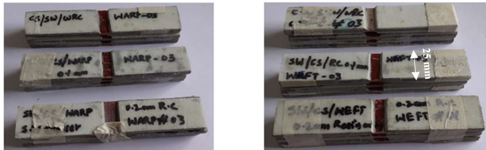
Fig. 6.31 Compressive test samples (warp and weft) with tabs (before testing)
