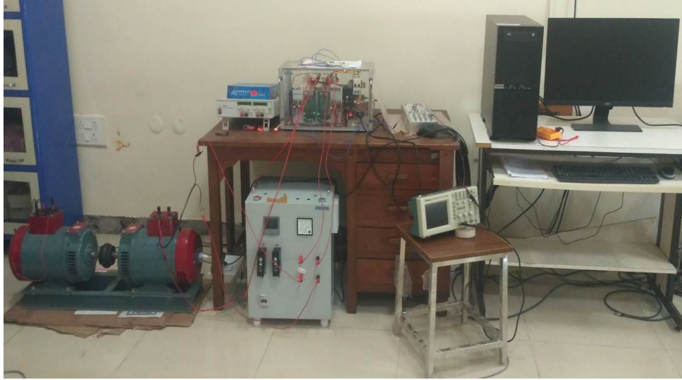
Figure 2.32 Real-time plant setup for DC motor speed control using FOPID controller
