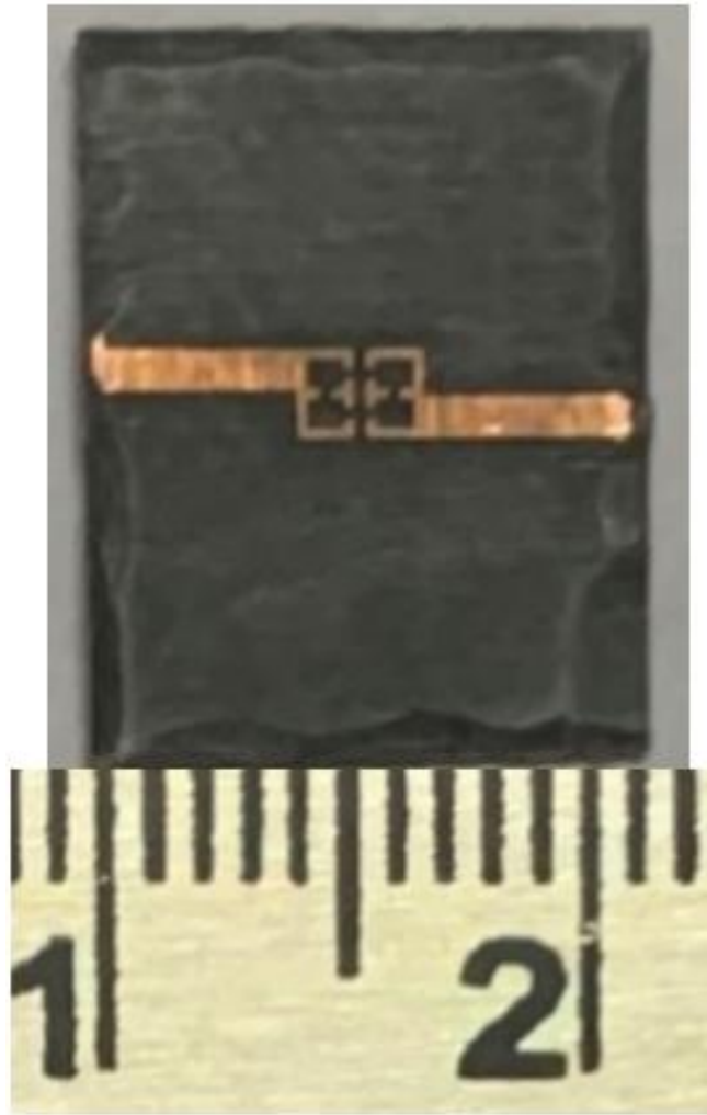
Fig 6.7 Top view of fabricated prototype for dual-split ring resonator dual bandpass filter
