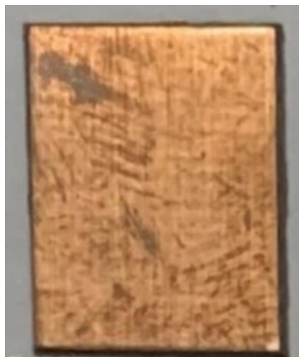
Fig 6.8 Bottom view of fabricated prototype for dual-split ring resonator dual bandpass filter
