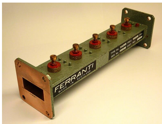
Fig 1.8 Five resonator waveguide bandpass filter
