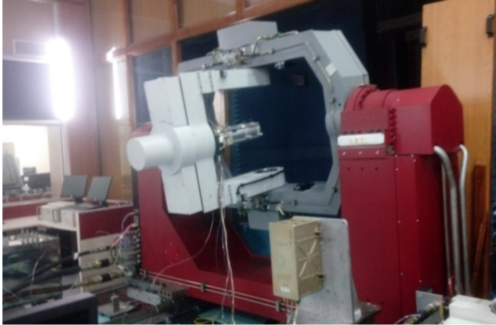
Figure 3.8 OBC-sensor-In-Loop Simulation testbed
