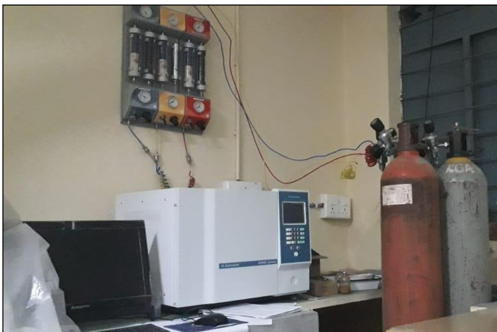
Plate. 3.3 Gas chromatography system for biogas analysis
