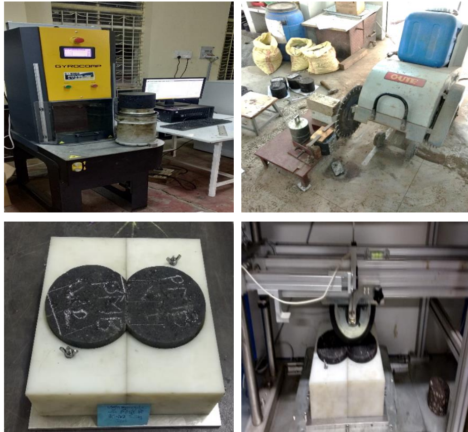
Fig. 3.16 Sample preparation for wheel tracking test
