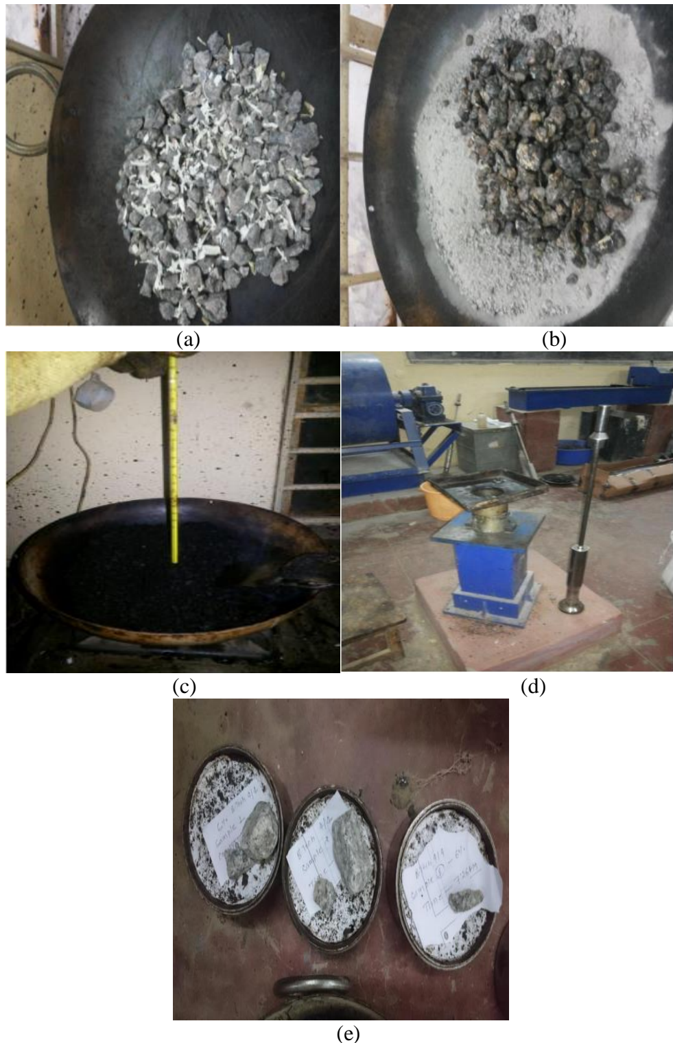
Fig. 6.3 Specimen preparation process for LBC mixtures: (a) preparation of LCA, (b) mixing of LCA with fine aggregate, (c) mixture preparation, (d) Marshall specimen compaction, and (e) compacted Marshall specimens
