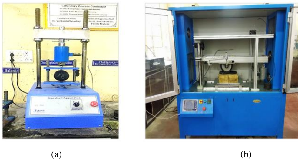
Fig. 3.4 (a) Indirect tensile strength test apparatus, and (b) wheel tracking device
