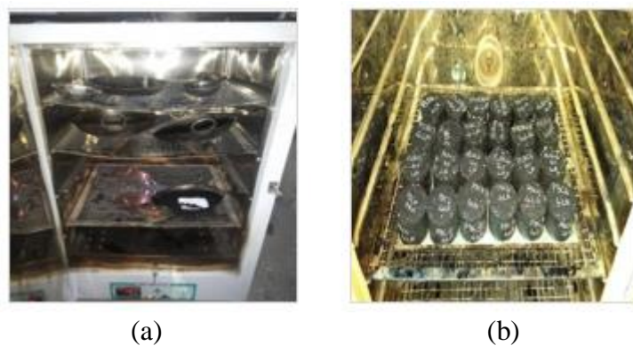
Fig. 3.7 (a) Short-term aging of bituminous mixtures, and (b) long-term aging of compacted bituminous mixture specimens
