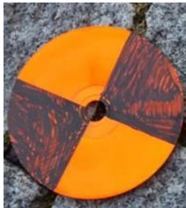
Fig 5.4 GCP marker placed on the ground for georeferencing
