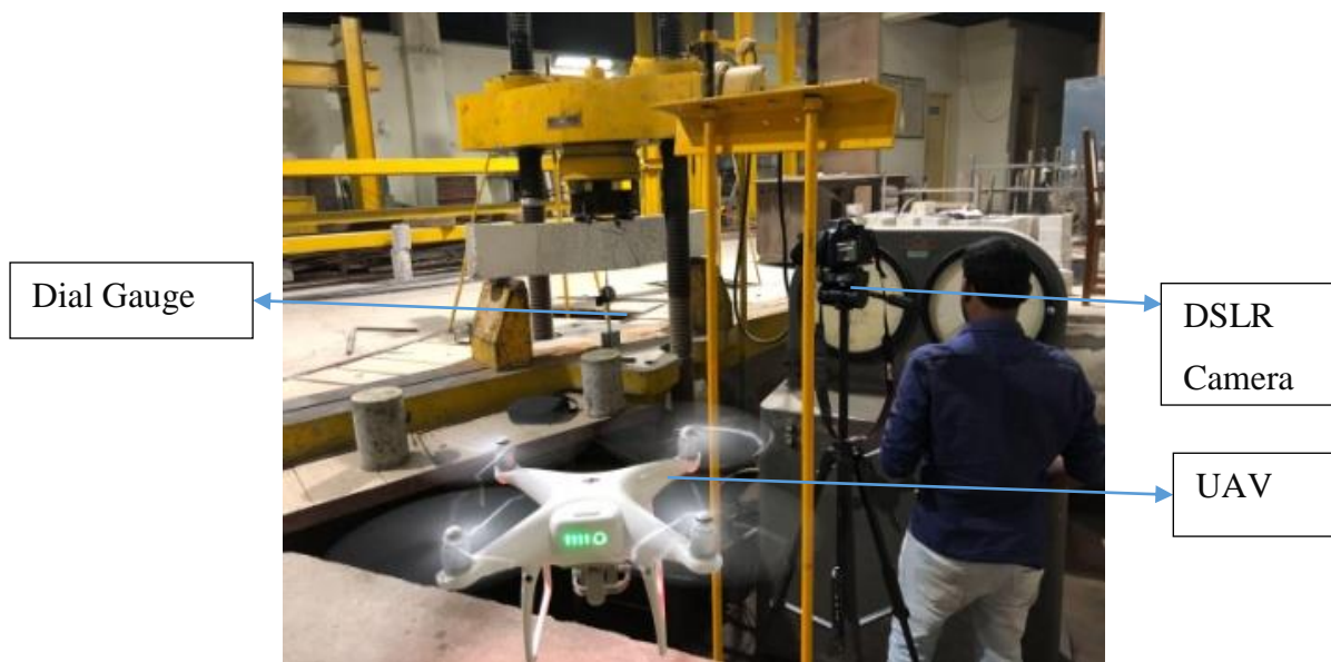
Fig 4.3 Loading test along with image acquisition using DSLR camera and UAV.
