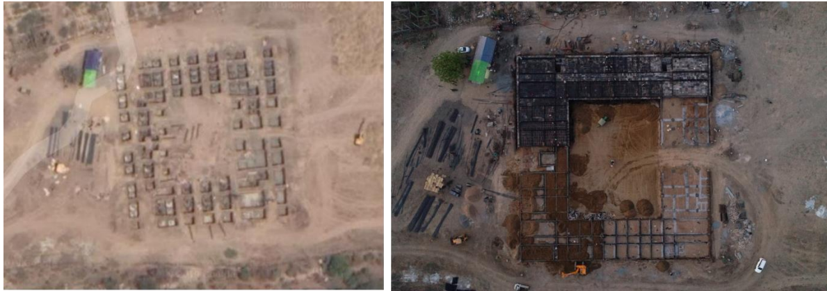
Fig 5.3 Drone image of construction site during foundation and plinth beam stages
