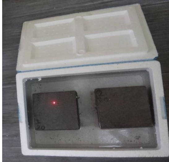
Fig 7.5 Concrete specimens for curing inside a polypropylene box.
