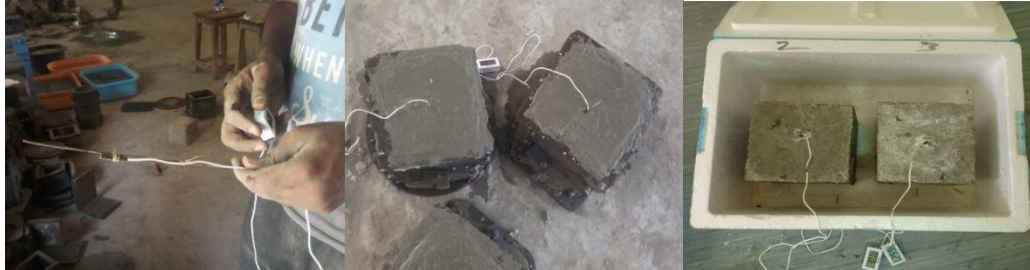
Fig 8.3 Thermocouple setup in concrete cube
