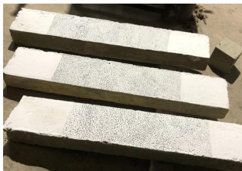
Fig 4.2Specimens preparation along with random speckle pattern
