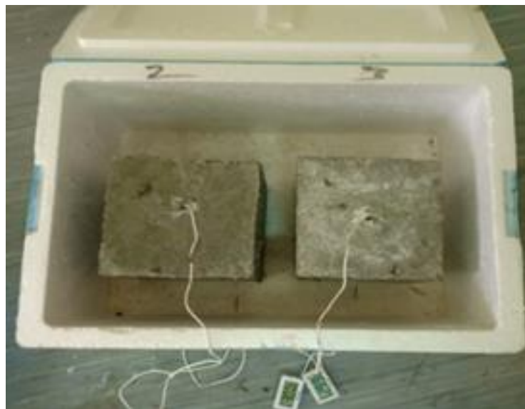
Fig 7.1 Thermocouple embedded concrete cube along with temperature displays
