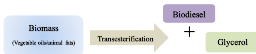
Scheme 2.1 Transesterification of biomass for bio-diesel and glycerol production.
