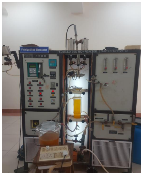
Figure 4.50 Fluidized bed Bioreactor used for biodegradation experiments
