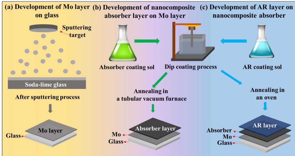
Figure 3.2.1. Schematic picture for the development of tandem absorber; development of (a) Mo layer, (b) nanocomposite absorber layer on Mo layer and (c) AR layer on nanocomposite absorber.
