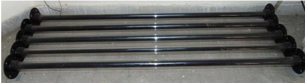
Figure 6.12. Digital image of a complete assembly of 2-m receiver tubes (4 Nos.) using commercially purchased Hi-min solar absorber tubes.
