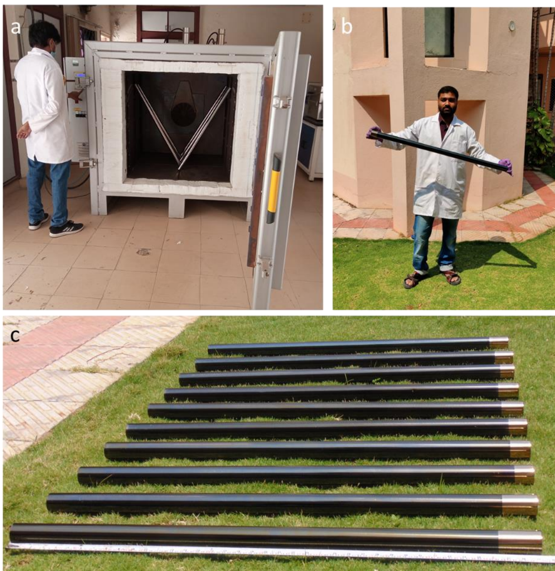
Figure 6.6. Absorber coated tubes in a large-scale furnace before annealing, (b) 1-m length absorber coated tube after annealing, and (c) display of 10 Nos. of absorber coated tubes.
