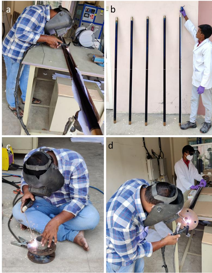
Figure 6.9. Assembling of 2-m prototype receiver tubes for field validation: Digital images of (a) joining the absorber tubes (1-m) by welding, (b) 2-m absorber tubes after welding, (c) and (d) assembling of absorber tubes with metal flanges and glass envelops.
