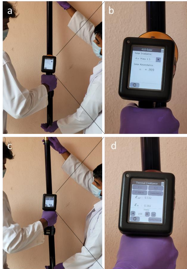
Figure 6.8. The digital image of measuring the (a, b) solar absorptance and (c, d) spectral emittance of tandem absorber tubes by 410-Visible / NIR portable reflectometer and ET-100 thermal handheld emissometer, respectively.
