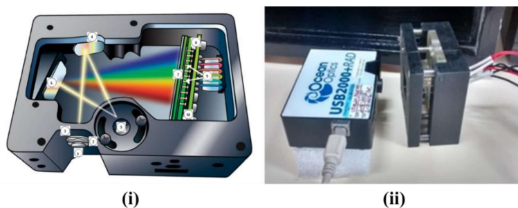
Fig. 2.15. (i) Schematic of light measurement process (adopted from Ocean Optics Operating Manual [113]) and (ii) photograph of spectroradiometer.
