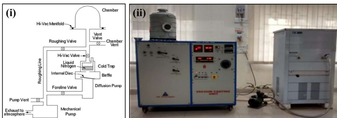
Fig. 2.4 (i) Schematic view of vacuum creating system and (ii) image of thermal evaporation vacuum coating unit with chiller system.
