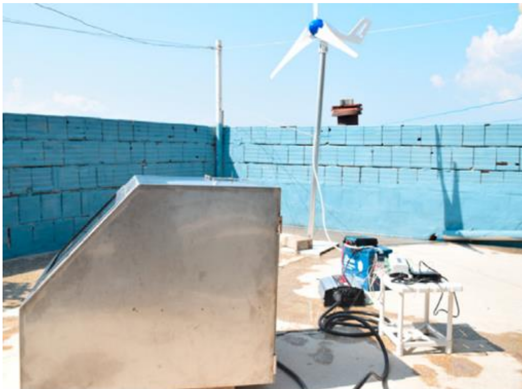
Fig. 2.4. Solar-wind hybrid type solar dryer [48]
