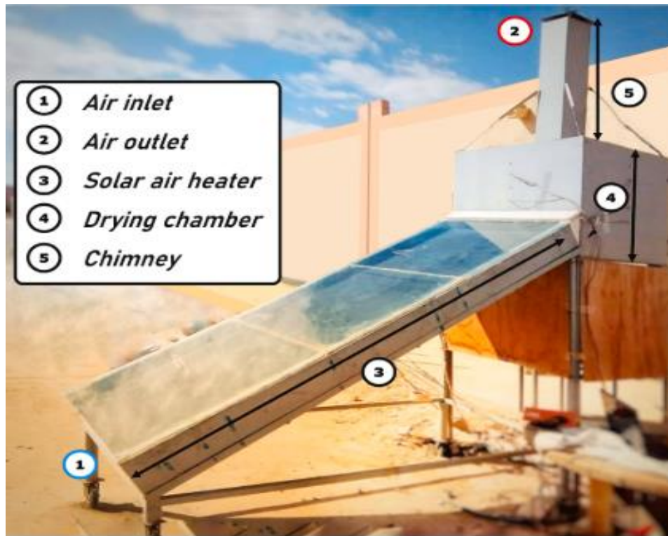
Fig. 1. 3. Indirect type solar dryer [18]
